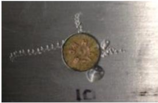
Figure 2: Typical drill bit damage incurred during removal of a steel ferrous fastener securing an aluminum lap-joint [11].
