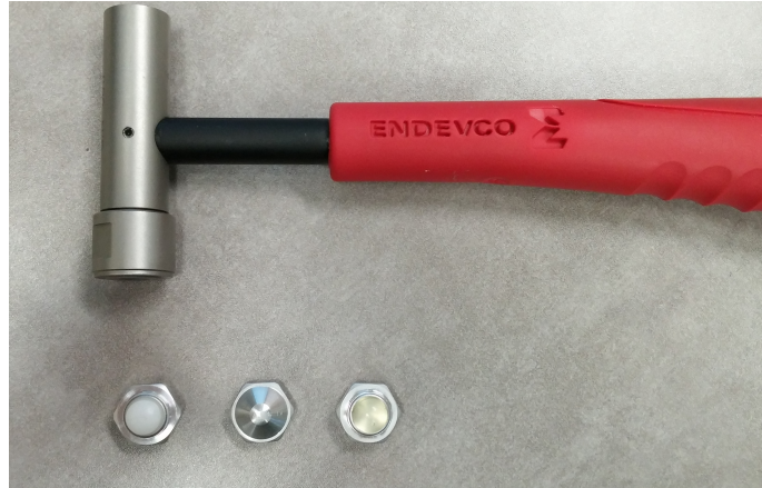
Figure 3.16: Endevco modal hammer and tips (from left to right, plastic, aluminum and rubber).
