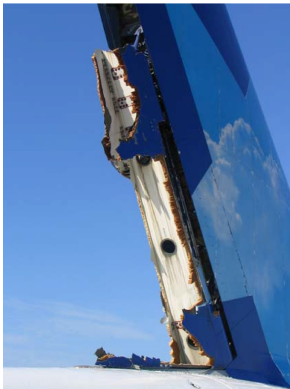
Figure 1.6: View of vertical tail plane and the remainder of the rudder from Air Transat Flight 961 [13].
