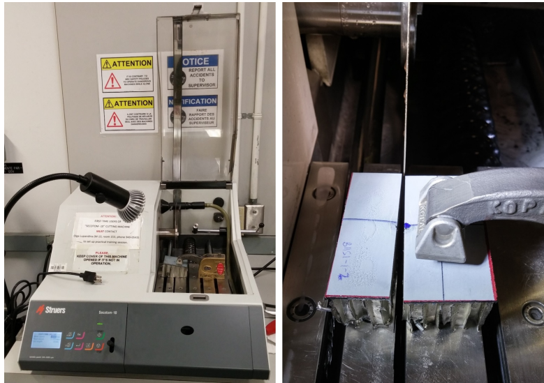
Figure 3.21: Specimen ready for sectioning (left) and sectioned and ready for damage characterization (right).
