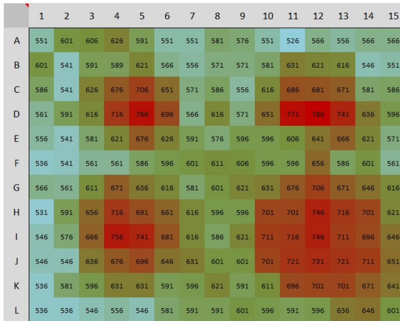
Figure 4.18: Local contact time map for B11 ( \mu s ).
