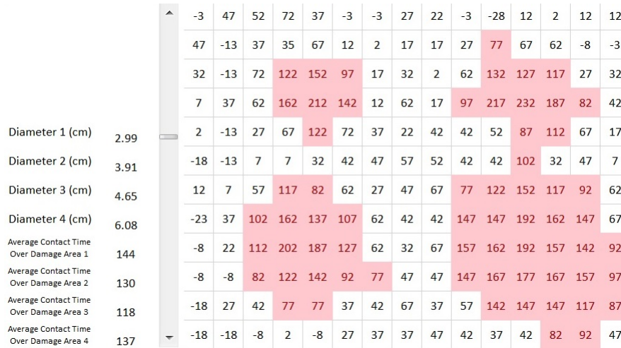
Figure 4.19: Damage map for B11 ( \mu s )
