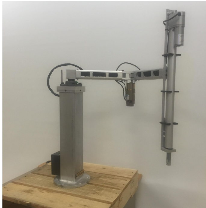
Figure 1.1: Photo of existing 3-DOF SCARA manipulator
