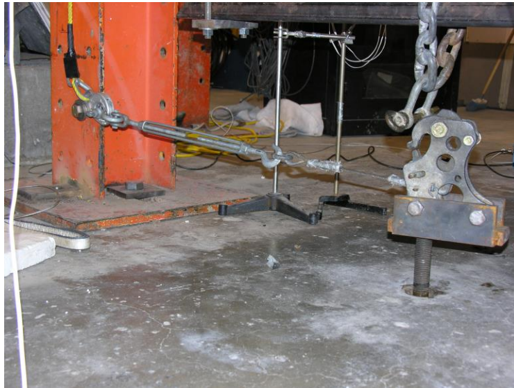
Figure 4-3: Release mechanism (before modifying chain mechanism)
