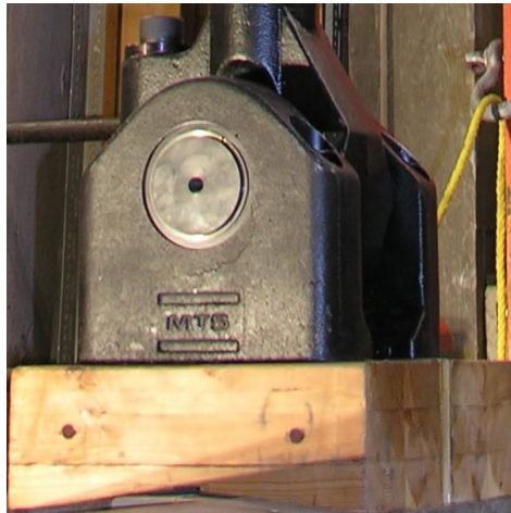
Figure 4-29: Actuator loading on dispersion block
