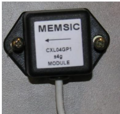
Figure 4-14: MEMSIC CXL04GP1 Accelerometer
