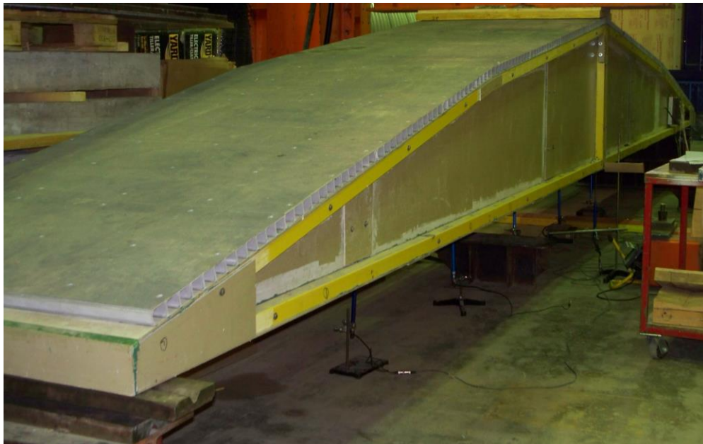
Figure 3-3: Experimental 10m GFRP bridge
