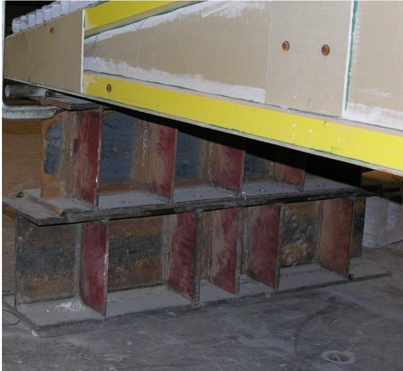
Figure 4-6: West End Support Pedestal
