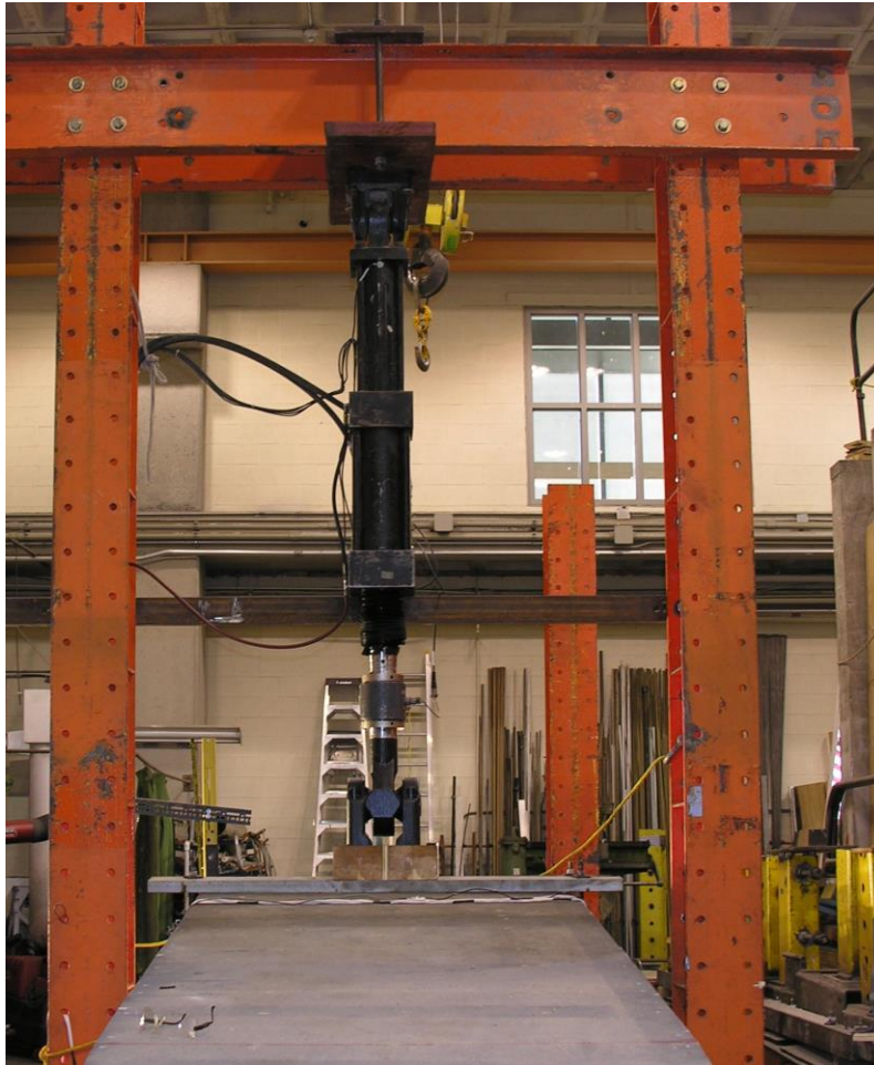
Figure 4-7: Actuator mounted in place on the support frame
