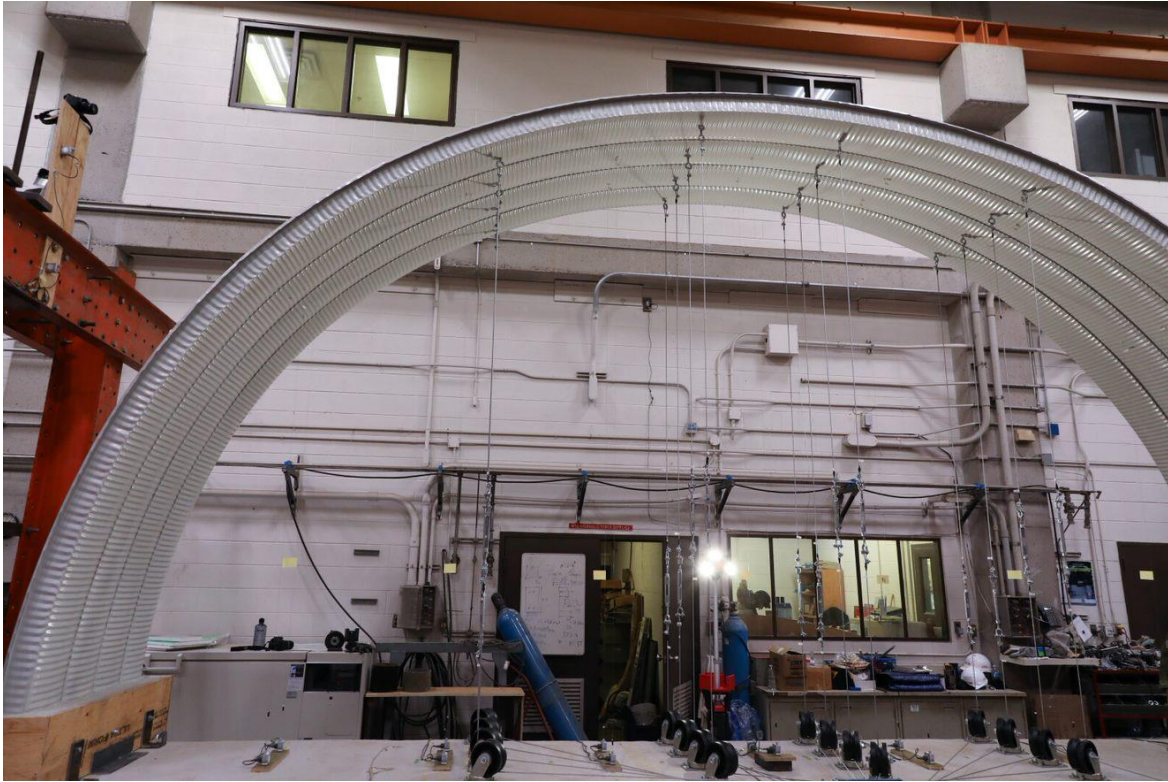
Figure C-23: Balanced Loading & Fixed Support Specimen Prior to Loading
