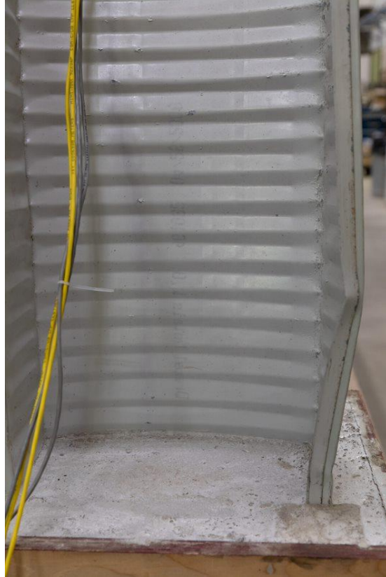
Figure C-25: Balanced Loading & Fixed Support Specimen Localized Buckling near Supports
