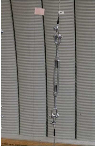
Figure 3-7: Turnbuckles Used for Adding Tension in Loading Assembly
