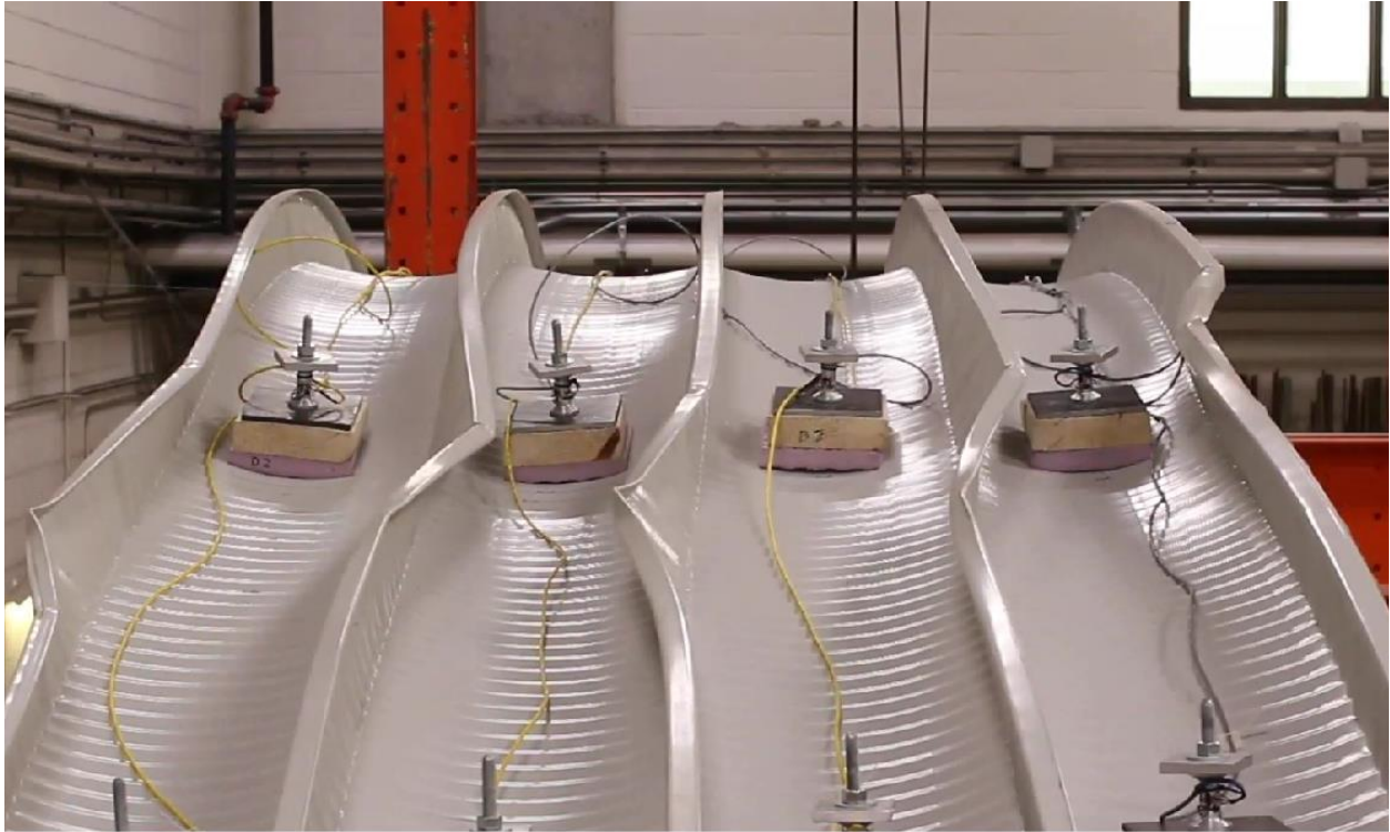
Figure C-43: Unbalanced Loading & Fixed Support Specimen Buckling of the Seamed Lips
