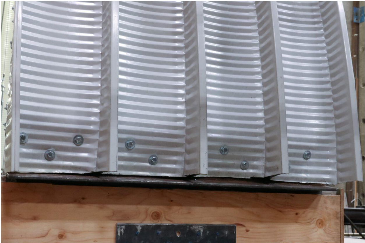
Figure C-46: Unbalanced Loading & Pinned Support Specimen Hinge Rotation Deformations
