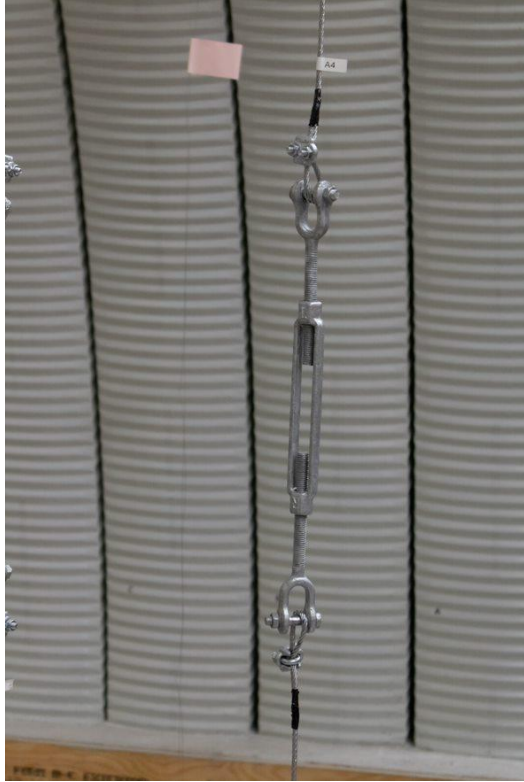
Figure C-13: Turnbuckles Used for Controlling Load on Cables
