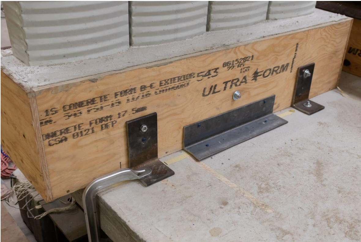
Figure C-20: Fixed Base Support 2
