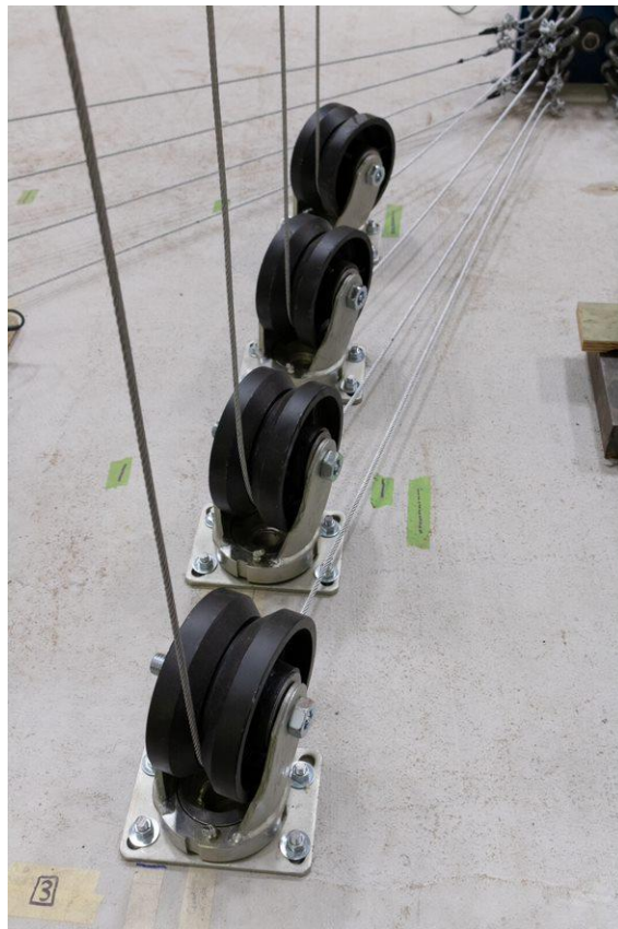
Figure C-12: Pulleys Anchored to Concrete Slab
