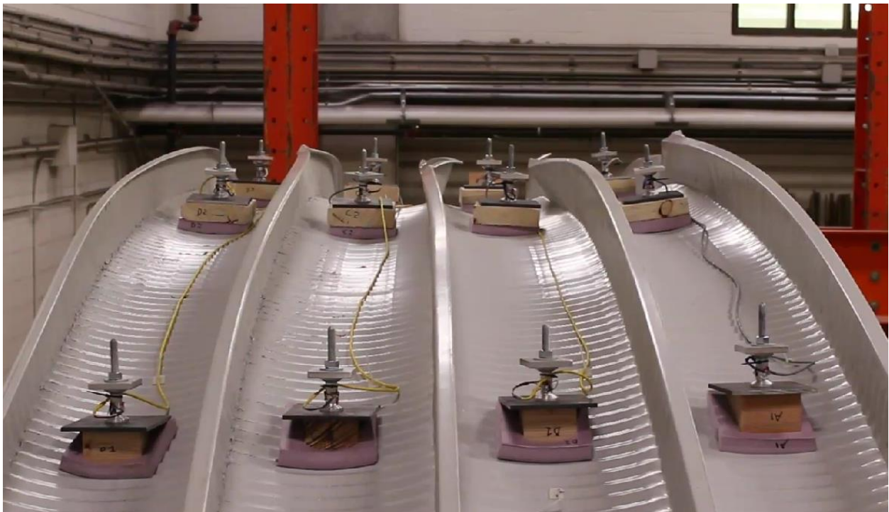
Figure C-30: Balanced Loading & Fixed Support Specimen Localized Buckling of Seamed Lips
