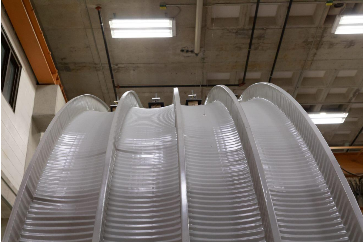
Figure C-41: Unbalanced Loading & Fixed Support Specimen Localized Web Deformations 1
