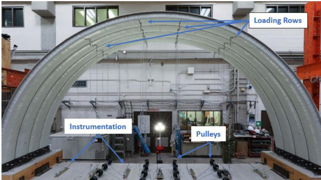
Figure 3-8: Pinned and Balanced Specimen Experimental Assembly
