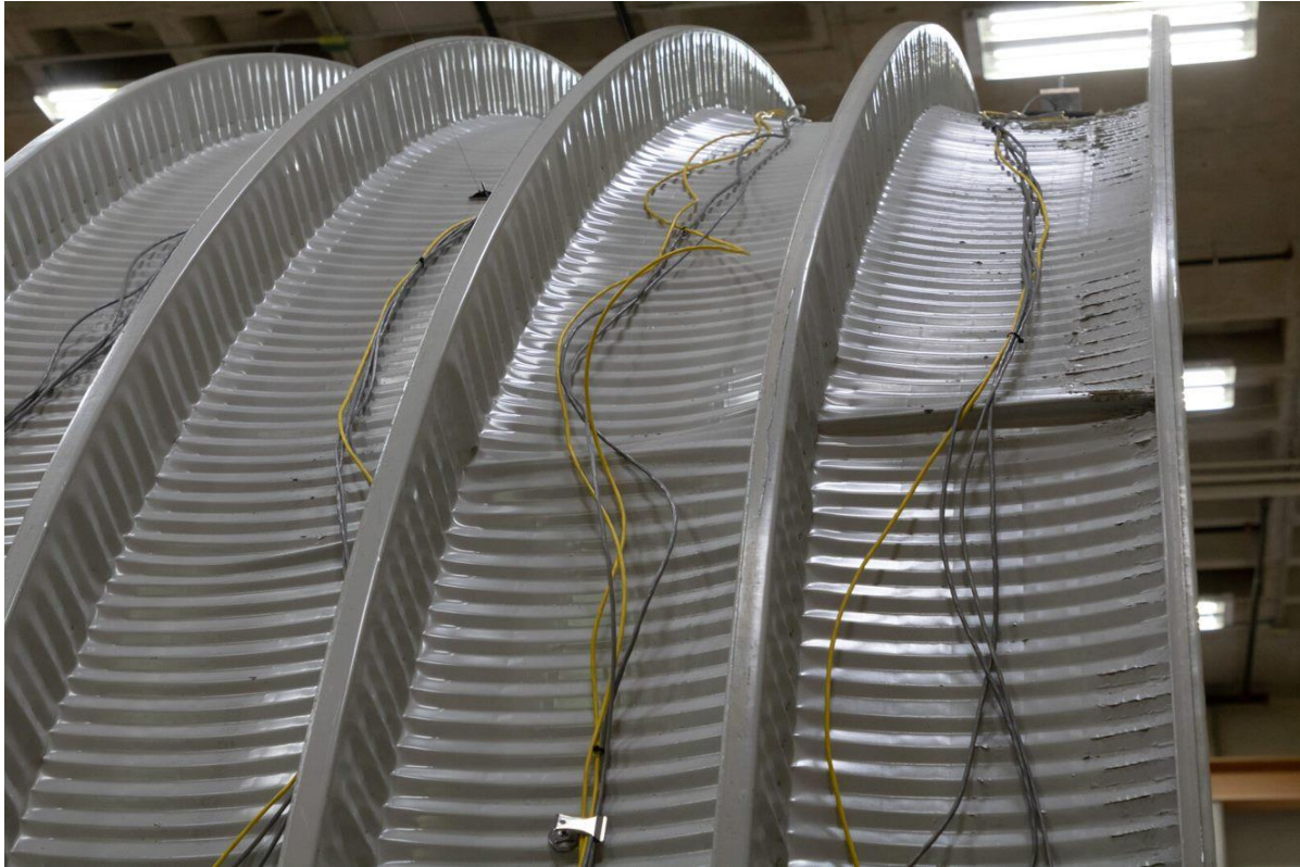
Figure C-37: Balanced Loading & Pinned Support Specimen Crimping of Webs Back Side
