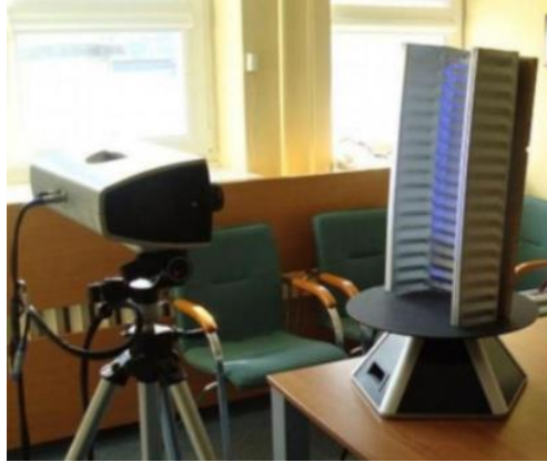
Figure 2-12: 3D Optical Scanning of Corrugated ABM-120 Panels [2]
