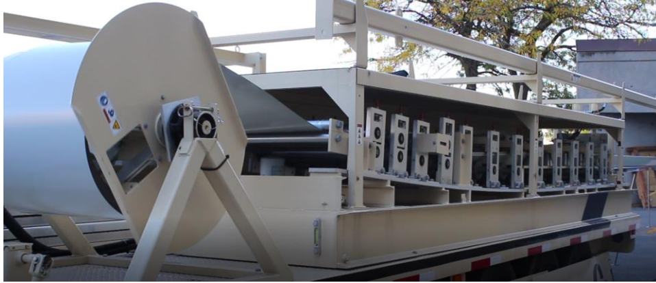
Figure 2-8: ABM Rolling Elements
