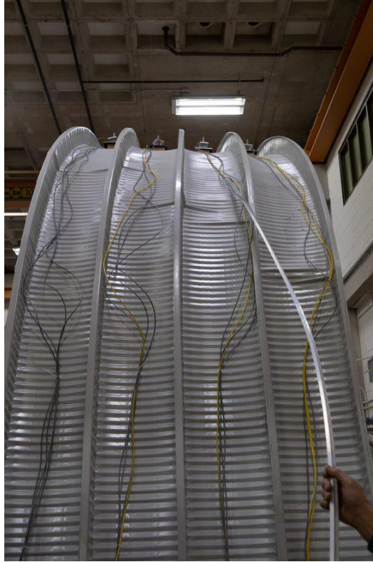
Figure C-27: Balanced Loading & Fixed Support Specimen Localized Crimping of Web from Back Side
