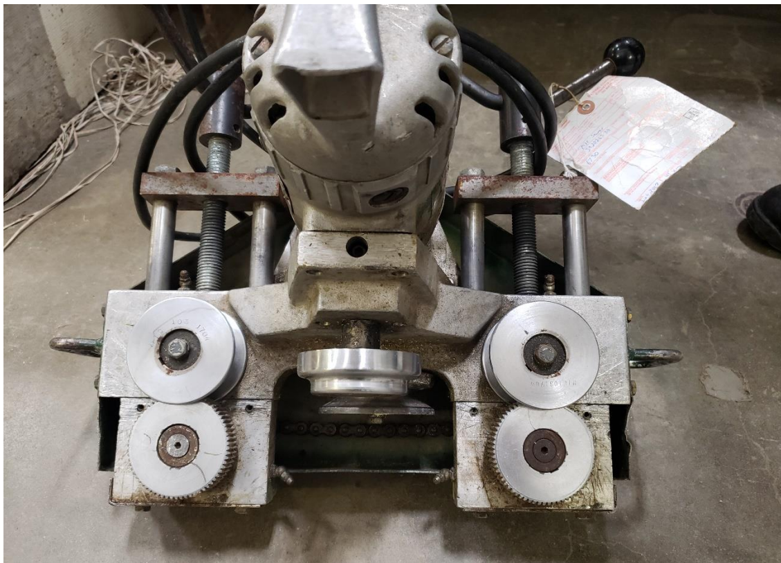
Figure C-6: Steel Rollers for Seaming Machine
