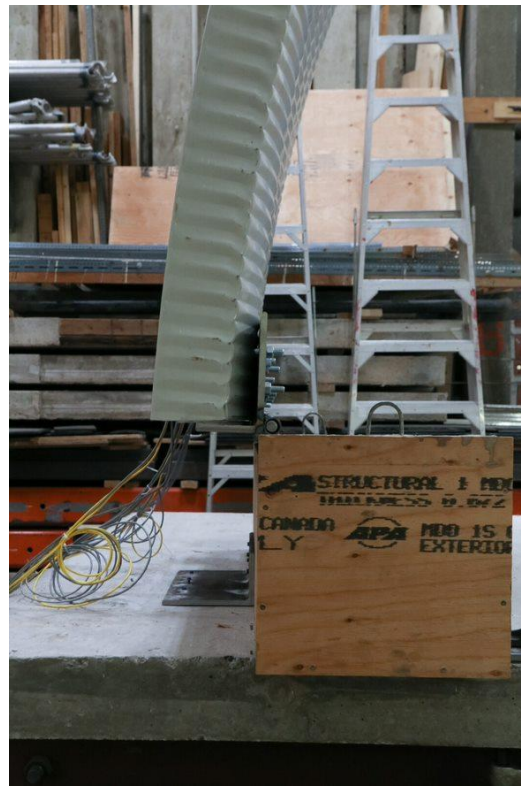
Figure C-22: Pinned Base Support 2
