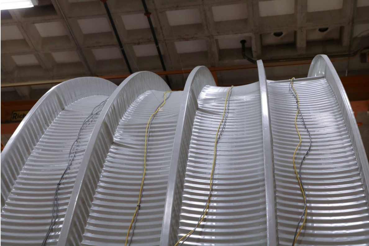
Figure C-47: Unbalanced Loading & Pinned Support Specimen Localized Web Crimping
