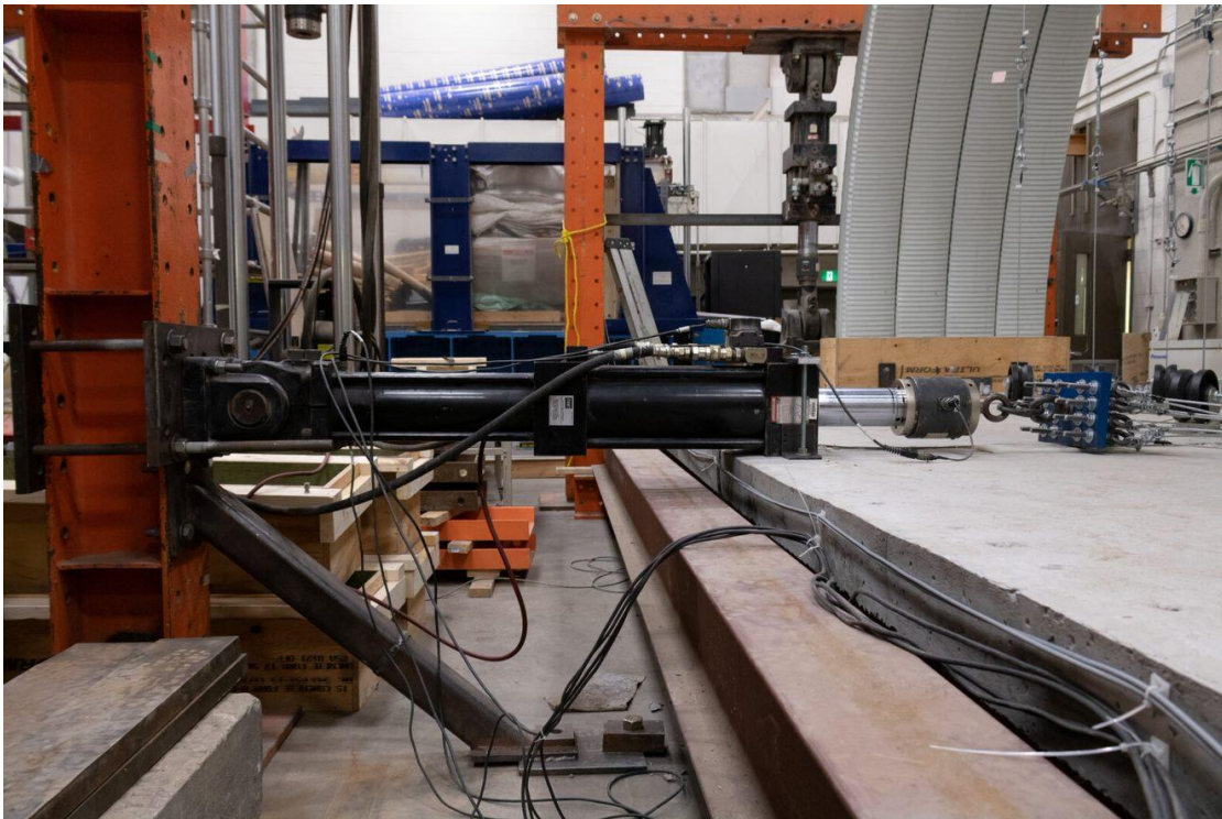
Figure C-10: 100 kN Actuator Set-up
