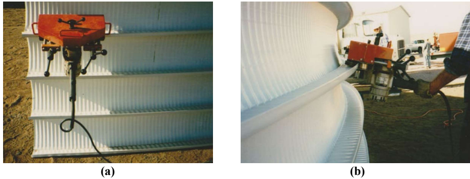
Figure 2.7 - Seaming machine (a) stationary and (b) in action [15]
