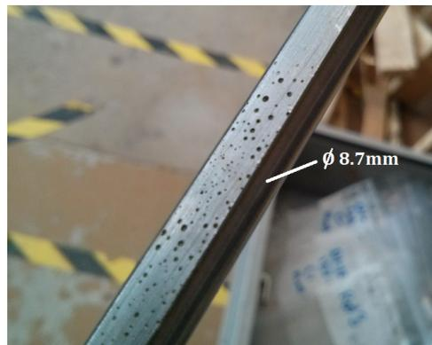
Figure 3.4: Visible surface-connected porosity on Galfenol rods.
