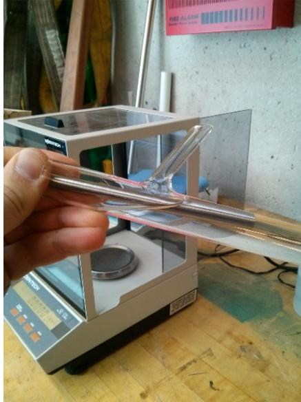
Figure A.3: Insertion of specimen for water displacement test.
