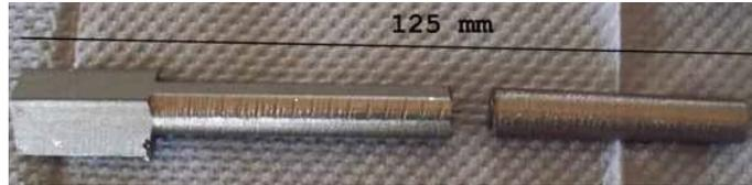
Figure 3.1: Brittle fracture of a 8.73 mm diameter cylindrical Galfenol rod machined from a quartered as-received sample.
