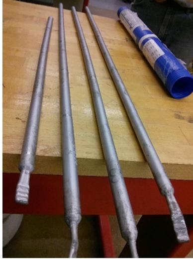
Figure 3.5: Encapsulated Galfenol rods as-received after HIP operation.
