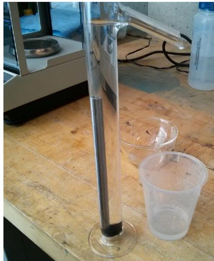
Figure A.1: Glassware used to perform water displacement tests.
