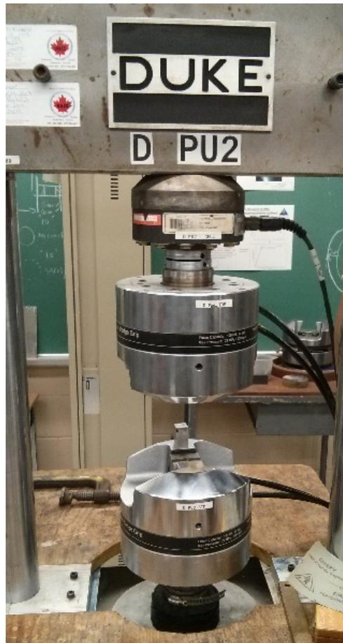
Figure 3.6: Electromechanical loading frame used for fatigue testing.
