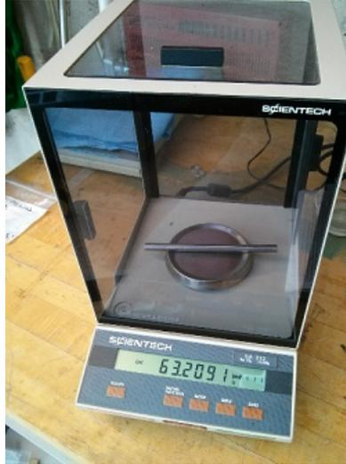
Figure A.2: Scale used to measure the weight of Galfenol rods and displaced water from submerged rods.
