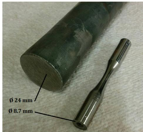
Figure 3.2: As-received Galfenol sample and fatigue specimen.
