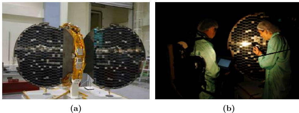
Figure 1.19: (a) The FORMOSAT III spacecraft arranged for optical ground truth characterization, and (b) determining the reflectance characteristics of the solar cells for an unspecified illumination and observation geometry. (Source: Abercromby, 2006)[21]
