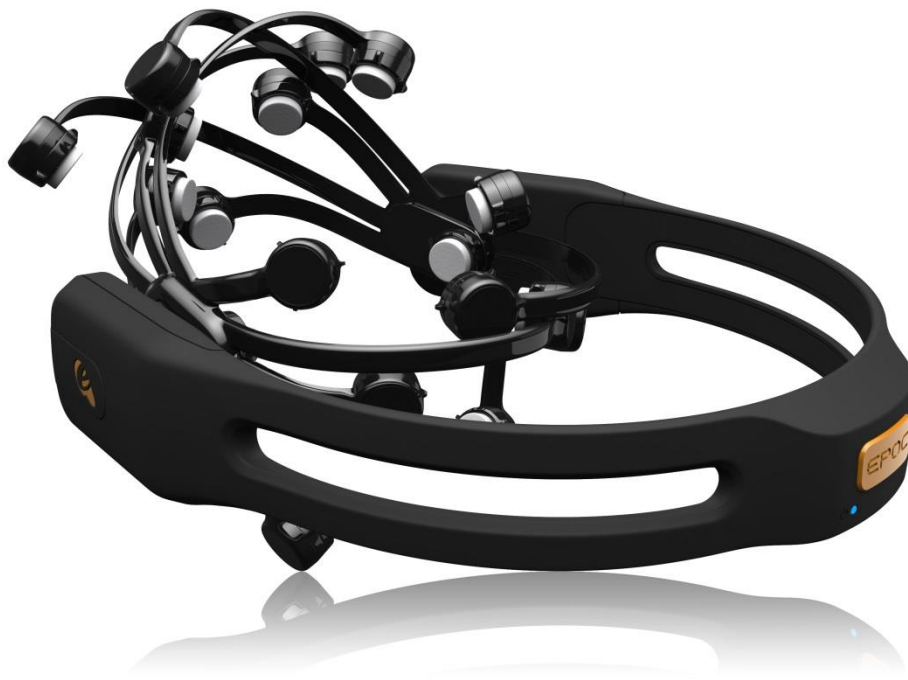
Figure 2: The Emotiv Epoc headset. This BCI device transmits 14 EEG signals at 128Hz via Bluetooth [21].
