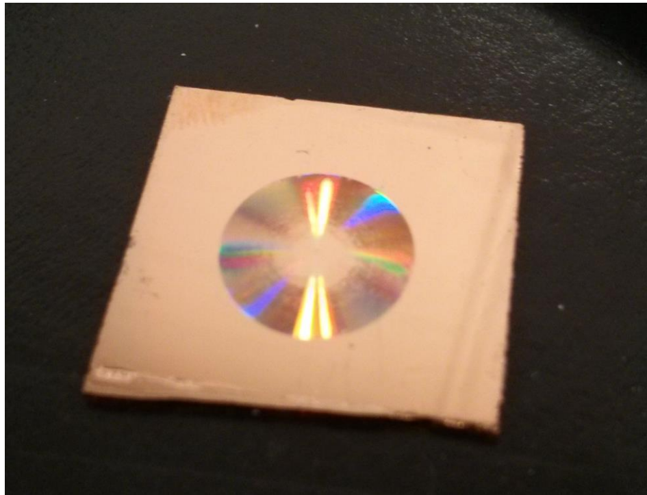
Figure 5.3 – A circular SRG with radius of approximately 11mm produced holographically using a CDG. This sample has been coated with gold prior to observations being made with a SEM. It can be seen that the grating pattern does not reach all of the way to the centre of the SRG, but forms a band of rings. This was done intentionally in order to ensure no cross over interference occurred from the opposite side of the CDG.
