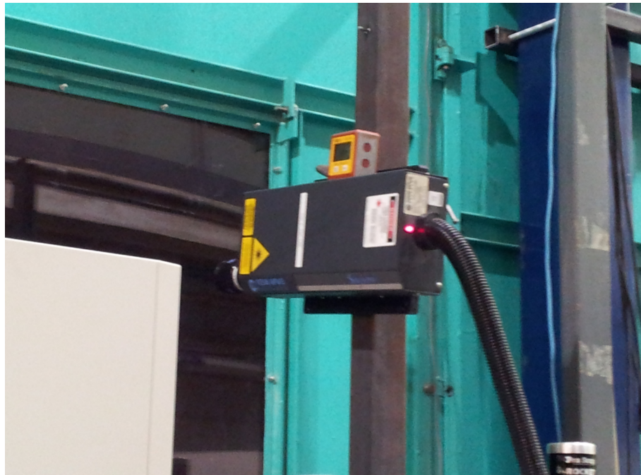
Figure 5.17: YAG Dual Cavity pulsed LASER
