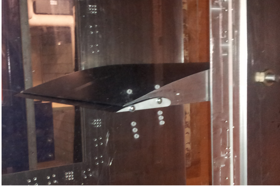
Figure 5.19: Clean configuration at 5° angle of attack
