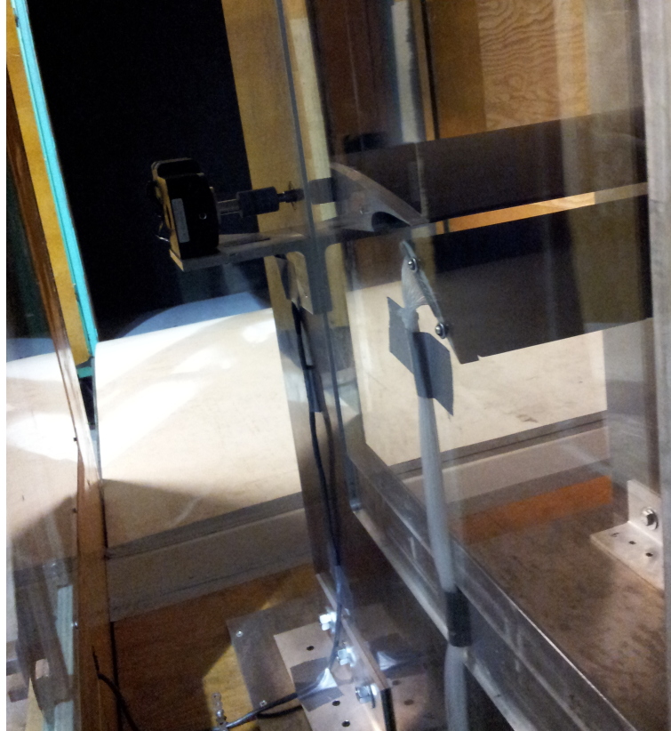
Figure 5.13: Stepper motor and Fowler flap pressure tubes
