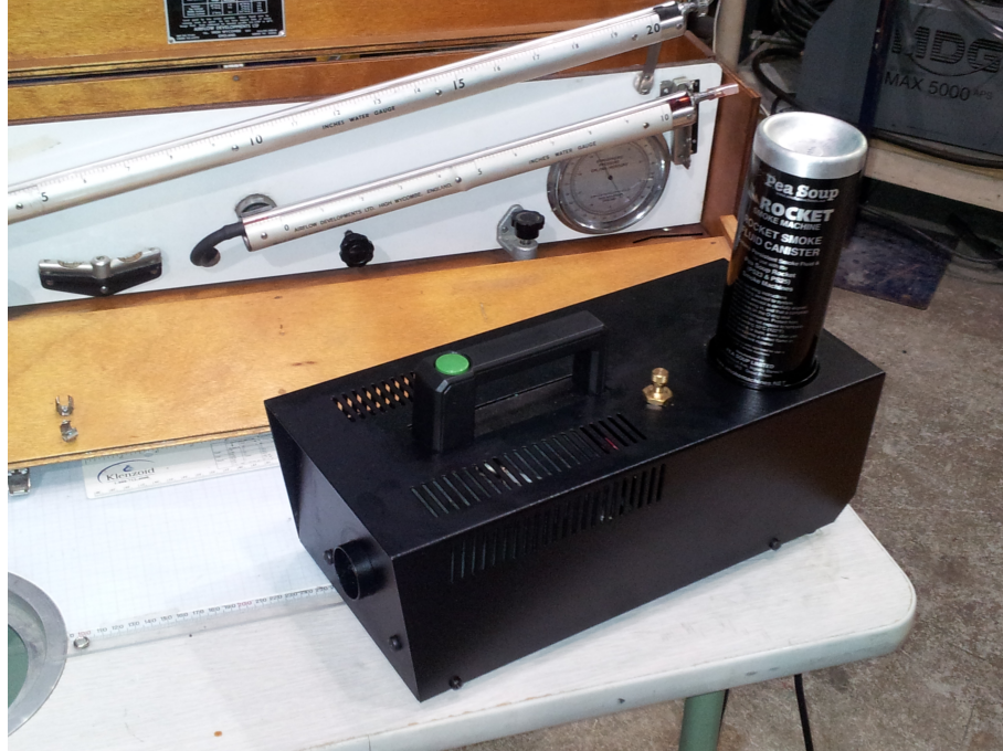
Figure 5.18: The Rocket smoke machine
