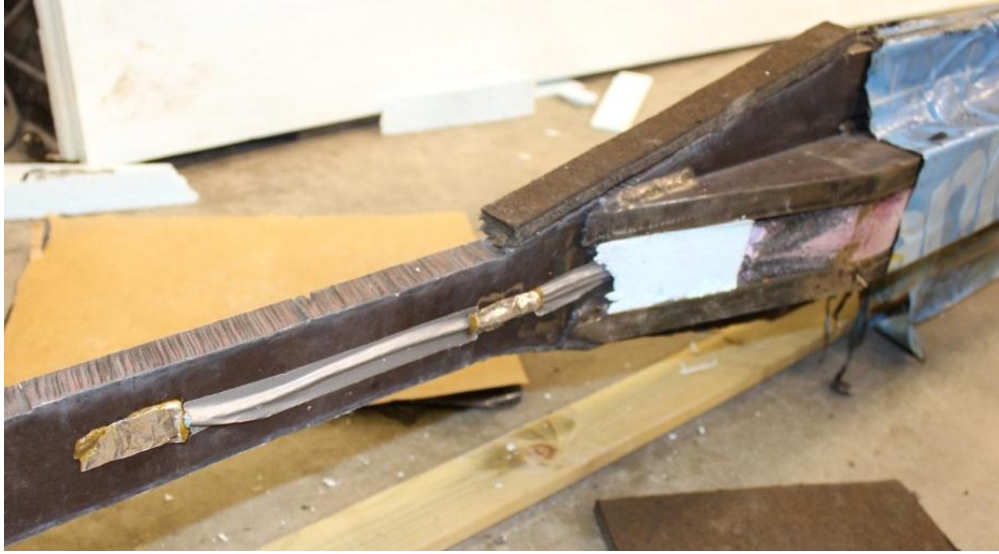
Figure 3.20 – Internal stain gauge and fibre board detail
