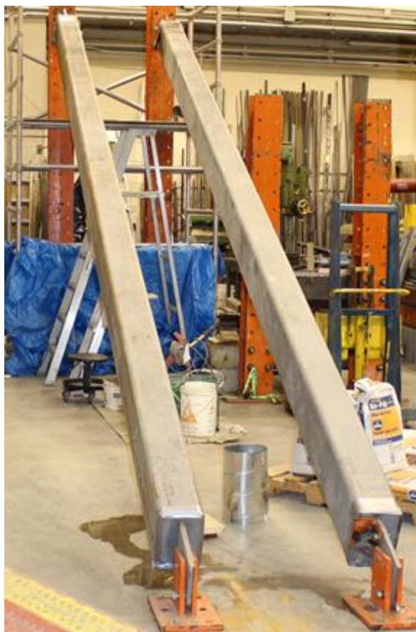
Figure 3.23 – Brace elevation for grouting
