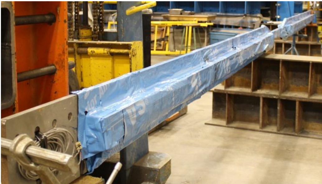
Figure 3.21 – BRB wrapped in un-bonding membrane
