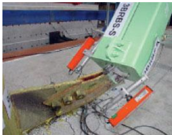
Figure 2.2 – Out of plane buckling (Della Corte et al., 2011)
