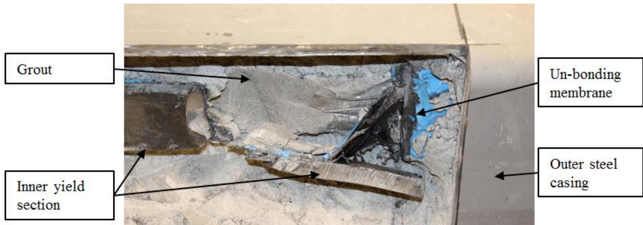
Figure 3.30 – Un-bonding membrane grout interface
