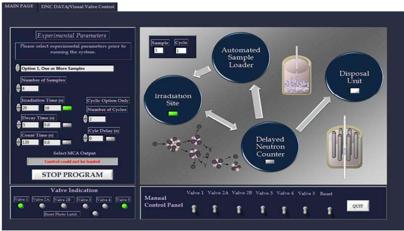
Figure 3.1: Delayed Neutron Counting System Graphic User Interface enables the selection of experimental parameters including irradiation, decay, count time, and number of cycles. Also includes a troubleshooting mode..
