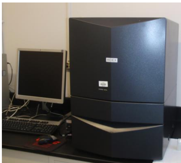
Figure A- 1. Hidex 300SL liquid scintillation counter
