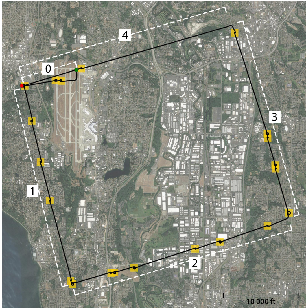
Figure 6.5: Thermal soaring SITL flight trajectory, with start marker (green), end marker (red), highlights of soaring events (yellow), and legs (white).
