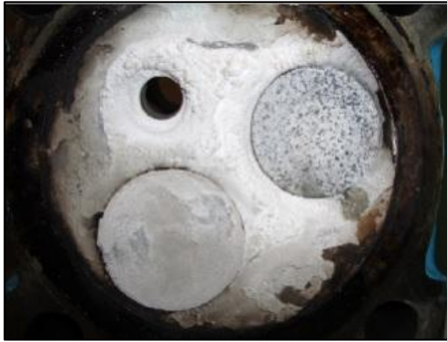
Figure 1.1.1. Cylinder head coated by amorphous silica deposits after 3500 hours of operation. Reproduced from Urban et al. (2009) [30].
