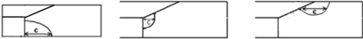
Figure 5.23: Illustrating the location of c for three initial crack locations.
