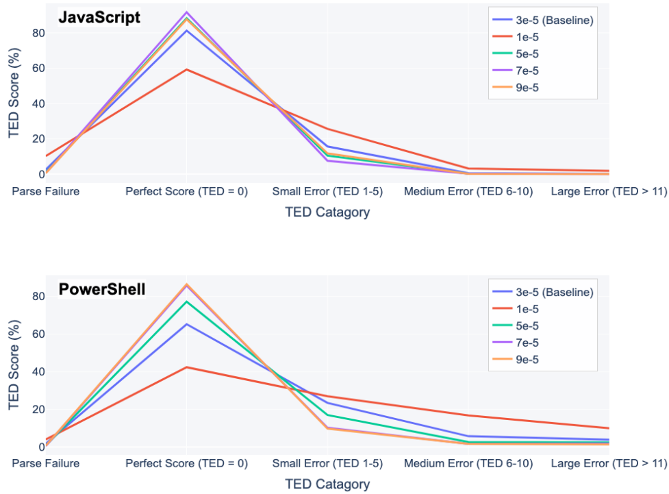
Figure 5.4: AST-T5 Hyperparameter Tuning Evaluation for JavaScript (top) and PowerShell (bottom), assessing the optimal learning rate during cross-language implementation.
