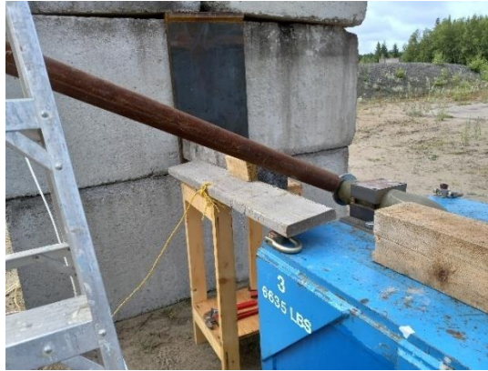
Figure 14. De-Fuzing of Projectile (Brassard, 2024)
