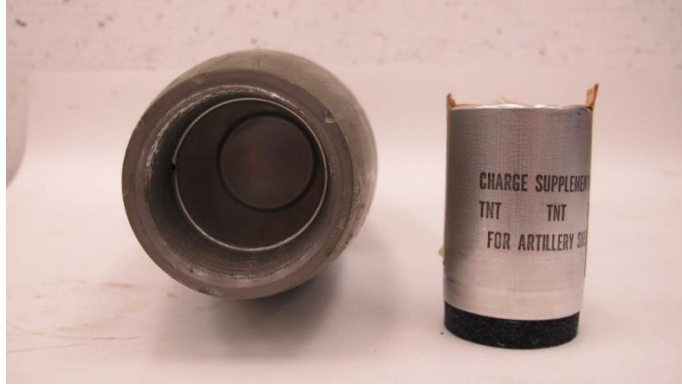
Figure 22. Booster Cavity and TNT Supplemental Charge
