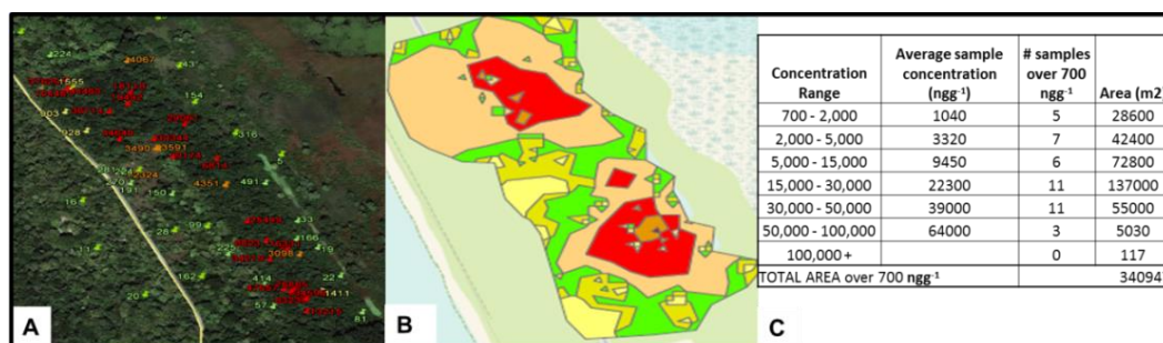
Figure 27. Middle section. A) All samples shown on Google Earth, and B) the corresponding interpolated ArcGIS. C) The mean, the number of samples, and area calculated for each concentration range.
