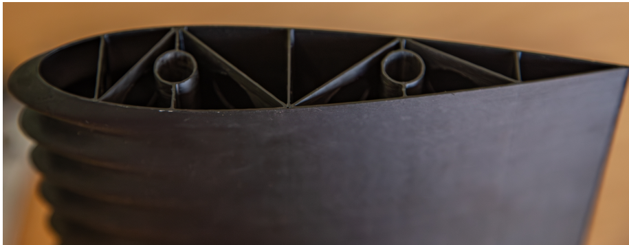
Figure 5.8: Cross-section of the 3D printed turbine blades used on the RMC VAWT.
