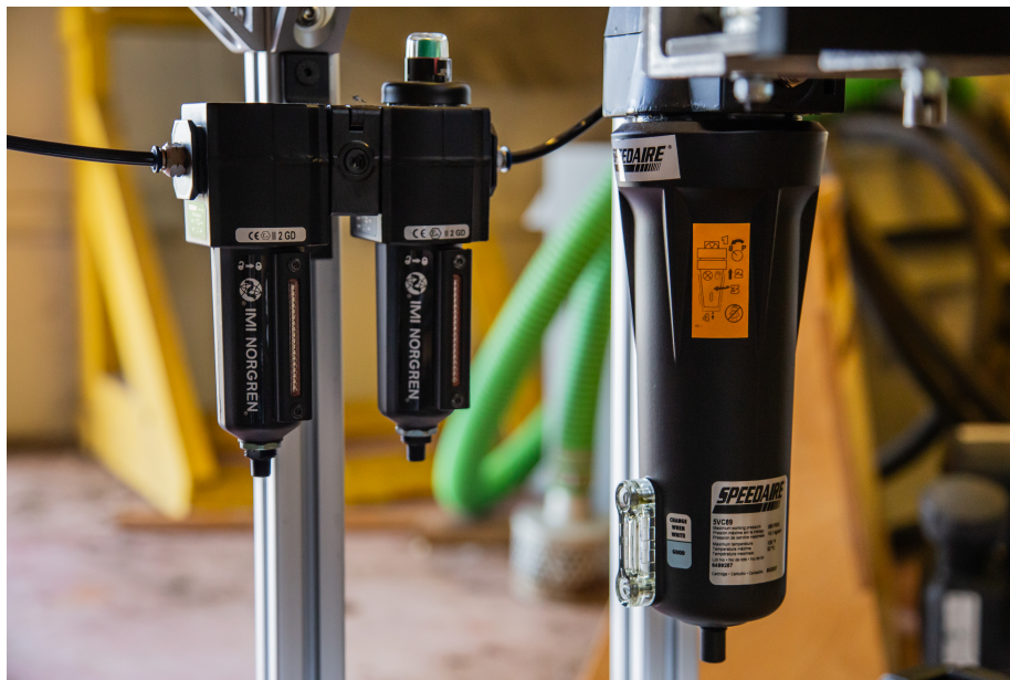
Figure 5.4: Air preparation filters and desiccant used for the air bearing on the RMC VAWT rig.
