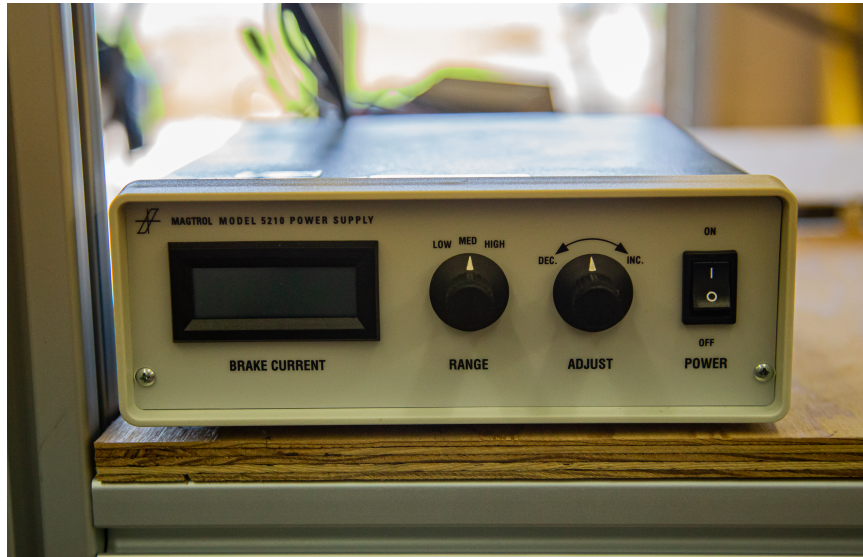
Figure 5.7: Magtrol 5210-2 power supply for the hysteresis brake.
