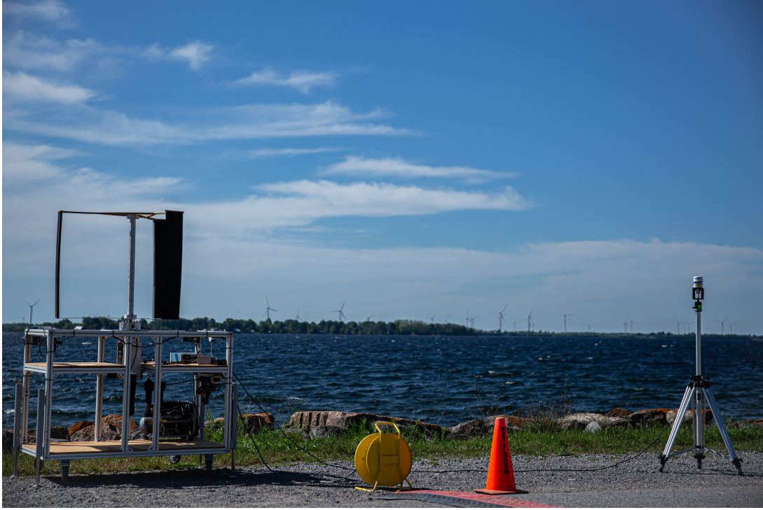
Figure 5.1: RMC VAWT setup during outdoor testing at the point of the RMC peninsula. The RMC VAWT Rig is on the left and the weather station is on the right.
