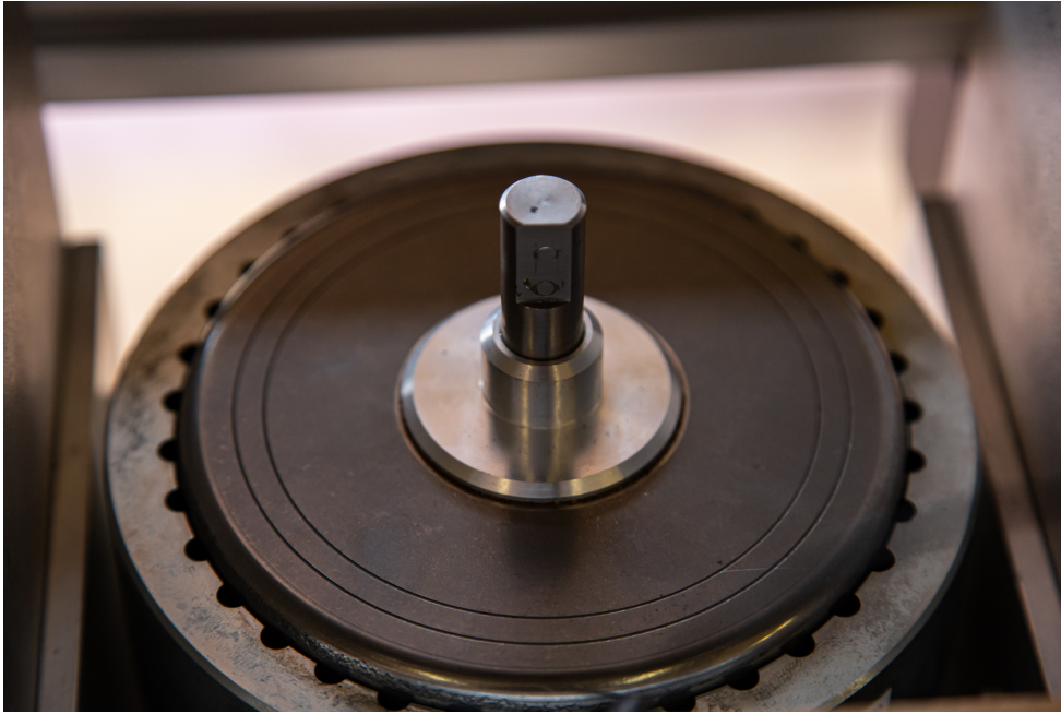
Figure 5.5: Magtrol HB-450 magnetic hysteresis brake on the RMC VAWT Rig.
