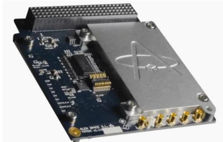
Figure 6.1 TOTEM SDR with wideband transceiver [121].
