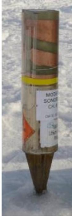
Figure 3.15 Geobuoy in Arctic ice [81].
