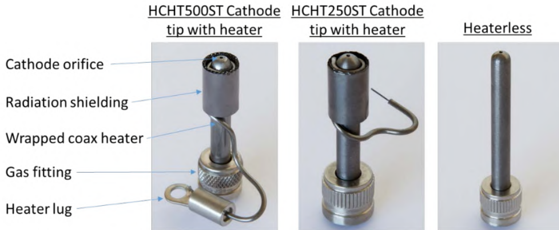
Figure 4.2.9: Hollow Cathode Tips from Plasma Controls LLC[83].
