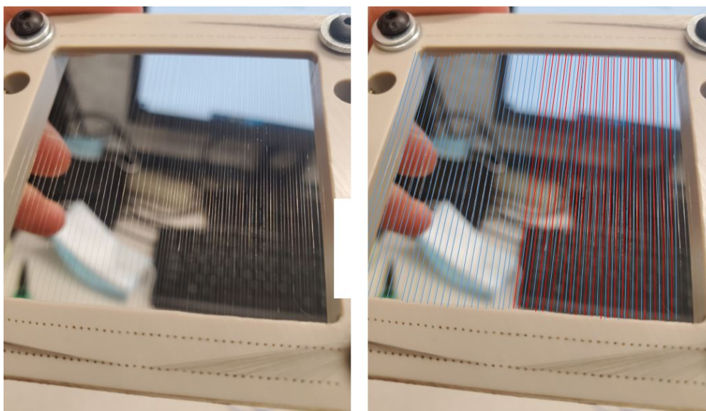
Figure 5.11: Bradbury Nielsen gate which is 75% of the tungsten wire threaded. RHS shows how the adjacent wires are isolated to different potentials (blue wires ground, red wires high voltage).
