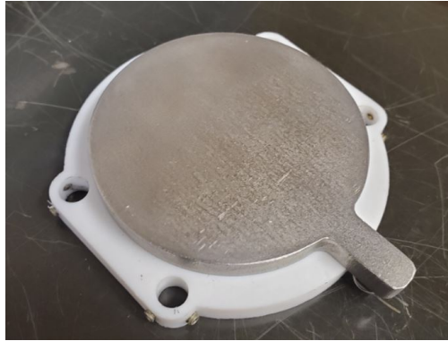
Figure 5.5: Electropray beam collector. A flat metallic plate surrounded by a Teflon frame.
