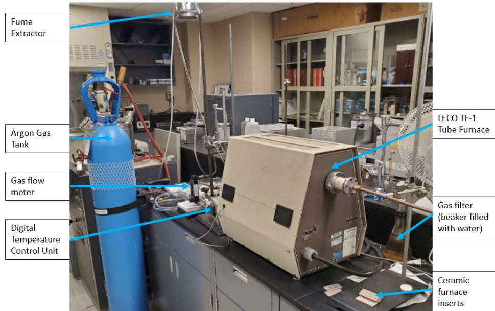
Figure A.2: Overview of the lab equipment used to pyrolyze the carbon xerogel samples.
