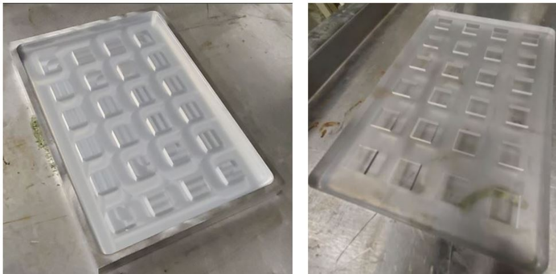
Figure 4.5: LHS The PDMS-b-PEO mold cooling in the aluminum mold. RHS - The stand alone PDMS mold.
