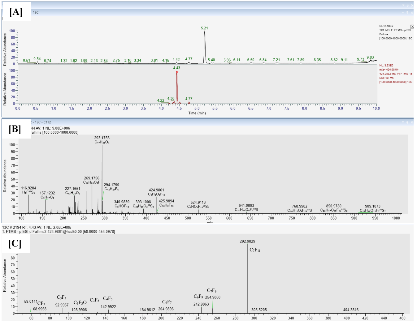
Figure A7: Chromatogram (A), spectrum (B), and ddMS 2 fragmentation (C) analysis of F/+CH 2 OH substituted PFOA following irradiation at 1 kGy, pH 7.
