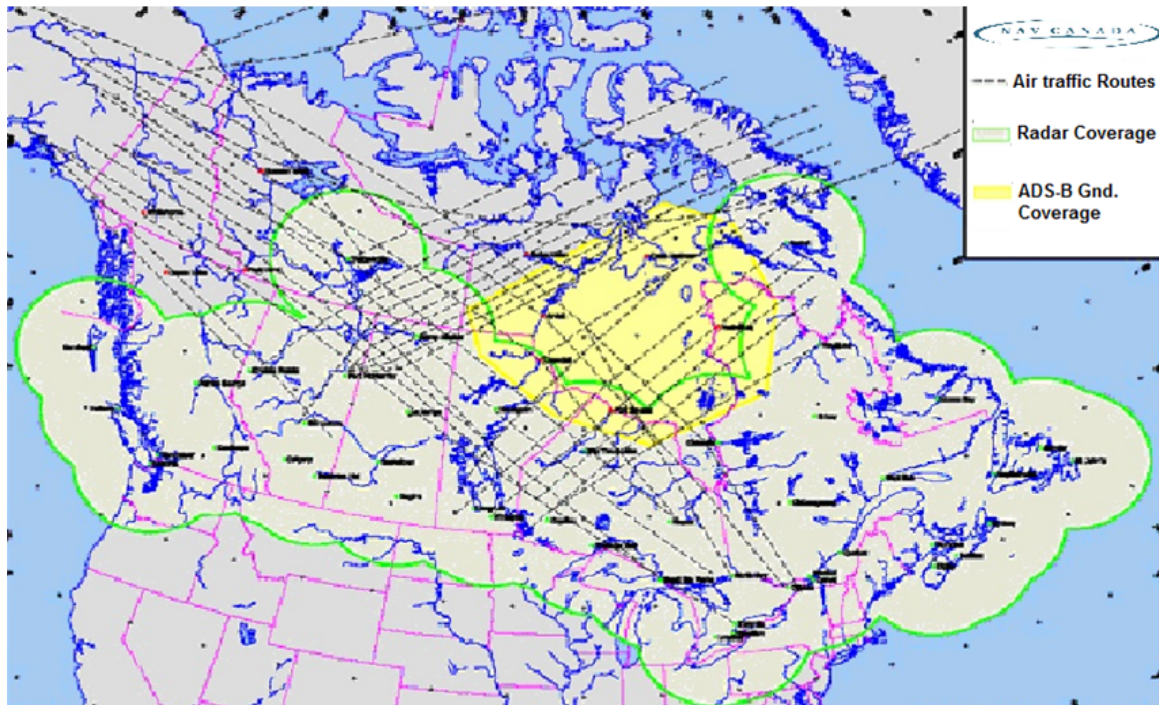
Figure 3.3: Nav Canada Radar (green) and ADS-B (yellow). Coverage reproduced from Nav Canada website: [NavCanada, 2011].
