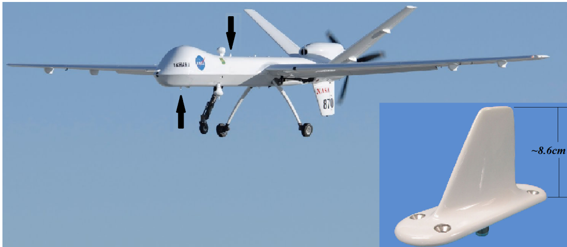
Figure 3.1: Main; shows Ikhana, NASA's unmanned ADS-B equipped aircraft test flight with the placement of two ADS-B antennas indicated by black arrows. Inset; shows the most widely adopted aircraft ADS-B antenna [Turner, 2012].
