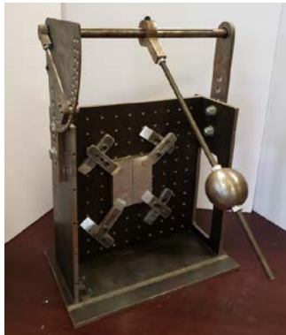
Figure 2-12: Pendulum apparatus used to impact the honeycomb sandwich panel coupons.
