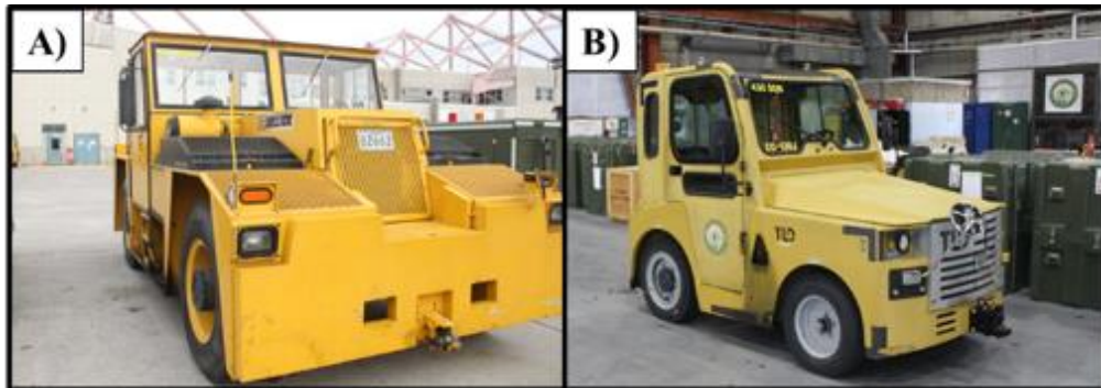
Figure 6.16: Aircraft Mobility Equipment A) Aircraft Tug, and B) Tow Tractor
