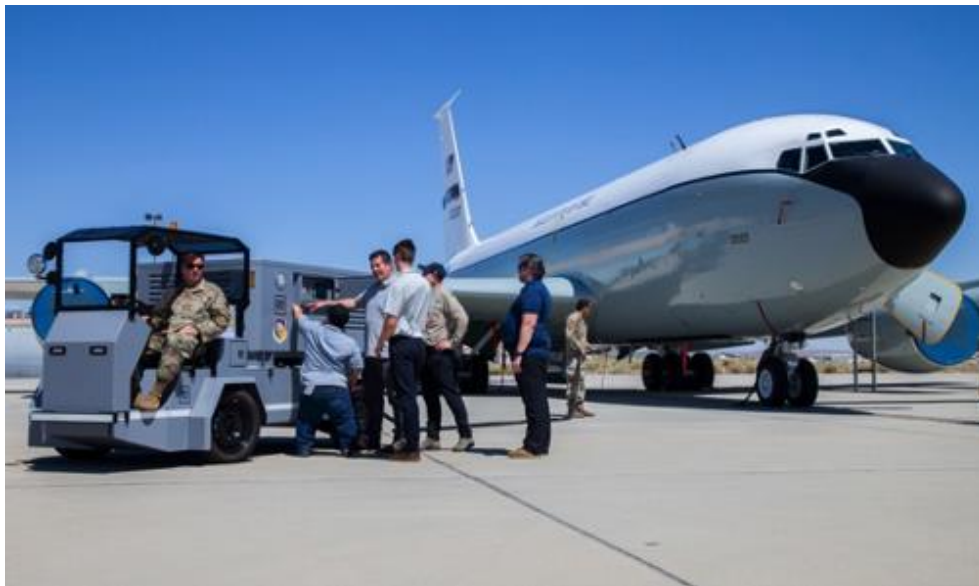
Figure 6.15: GM Defense’s Electric GPU at Edwards Air Force Base (Air Force Research Laboratory Public Affairs, 2023)
