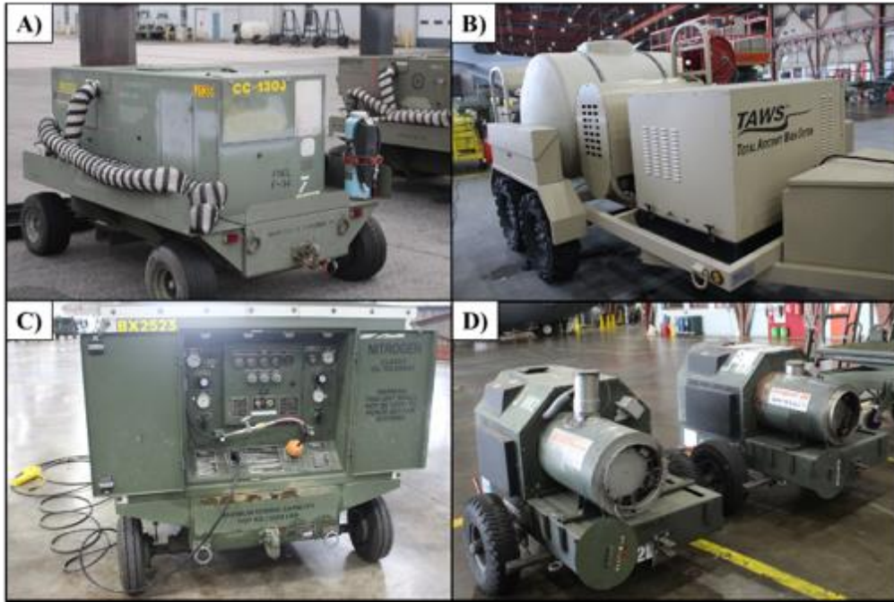
Figure 6.17: Aircraft Servicing Equipment A) Combined Services Unit, B) Aircraft Wash, C) Nitrogen Servicing Cart, and D) Heater Cart
