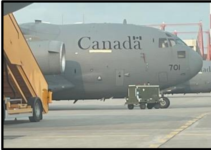
Figure 6.13: CC-177 with GPU
