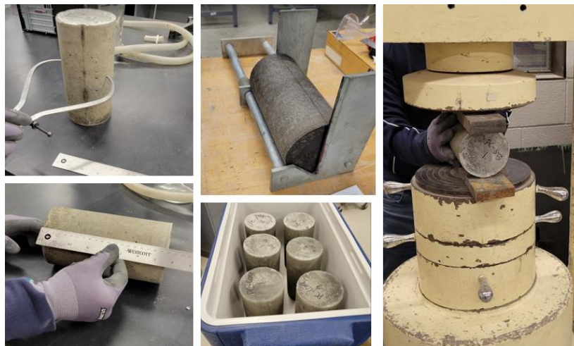
Figure 3-9. Preparation measurements and STS testing setup
