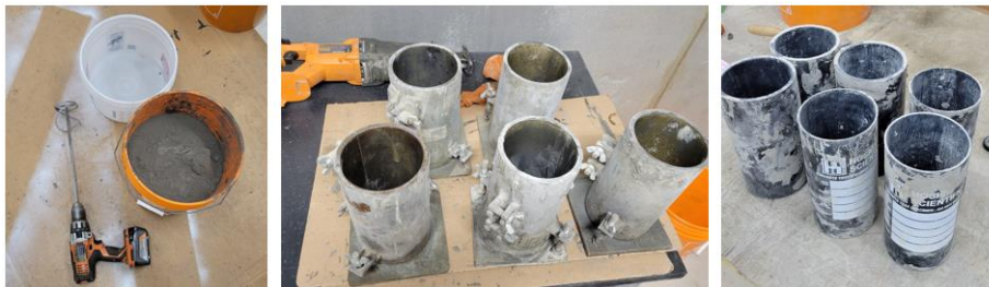
Figure 3-28. Water-cement mixing and cleaned/oiled moulds
