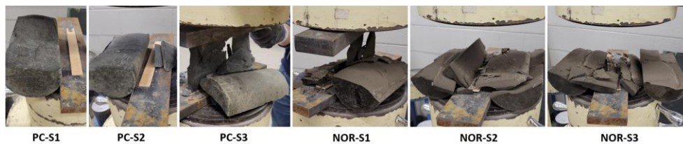
Figure 3-10. Tensile testing of grout cylinders
