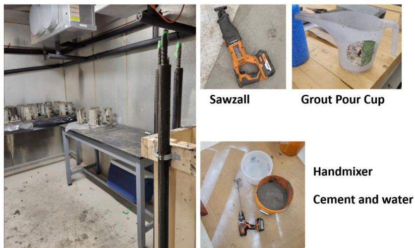
Figure 4-10. Grouted specimens and test cylinders in freezer room; grouting tools
