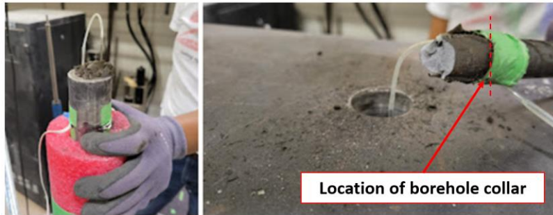
Figure 4-34. P5-90 specimen rebar tensile failure inside of embedment length, green tape marks location of borehole collar
