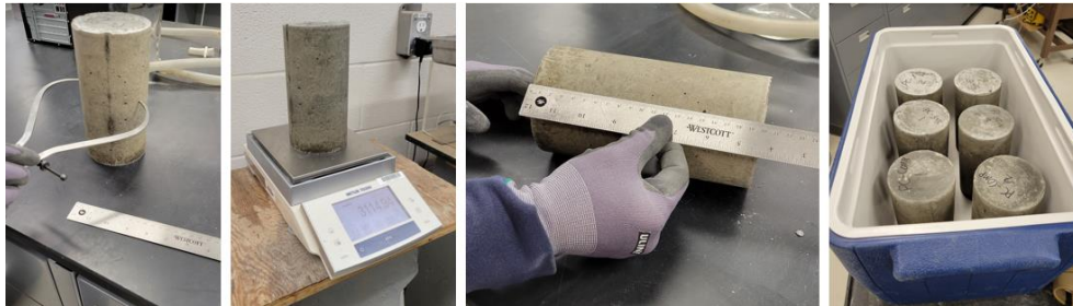
Figure 3-6. Pre-test grout cylinder measurement process
