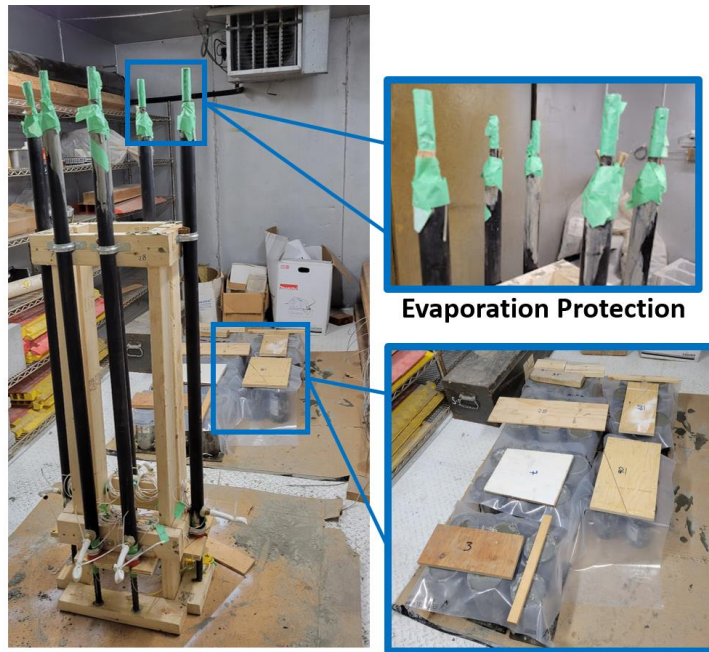
Figure 5-8. Evaporation protection of FGRB specimen ends and grout cylinders
