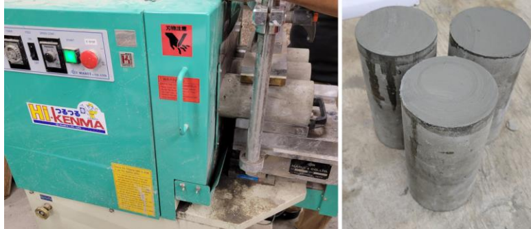
Figure 3-4. Preparation of UCS cylinders using grinding machine
