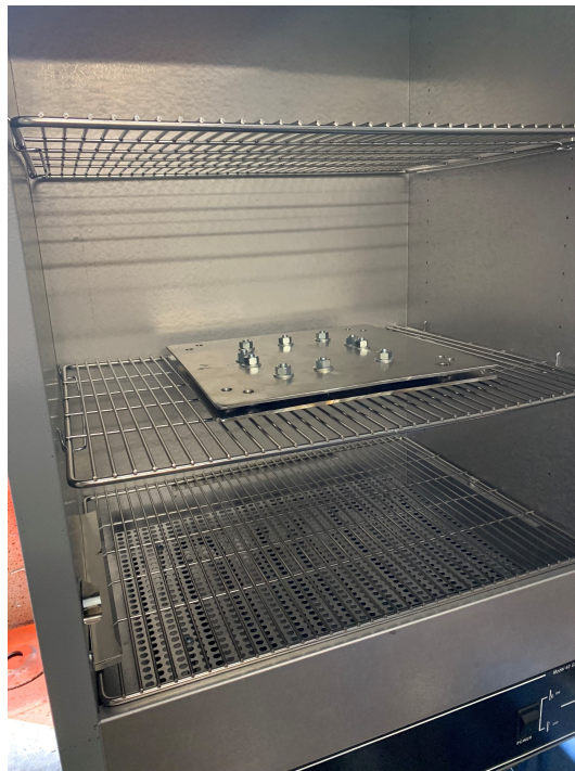
Figure A.6: Antenna 1 in fabrication oven
