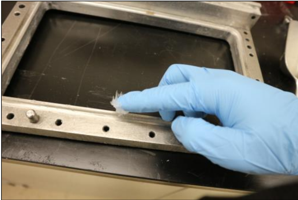
Figure D-15: Applying grease in bottom track of the other cradle side plate.
