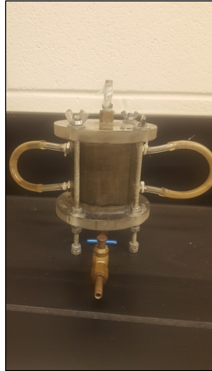
Figure B-3: Permeameter used for constant head testing.
