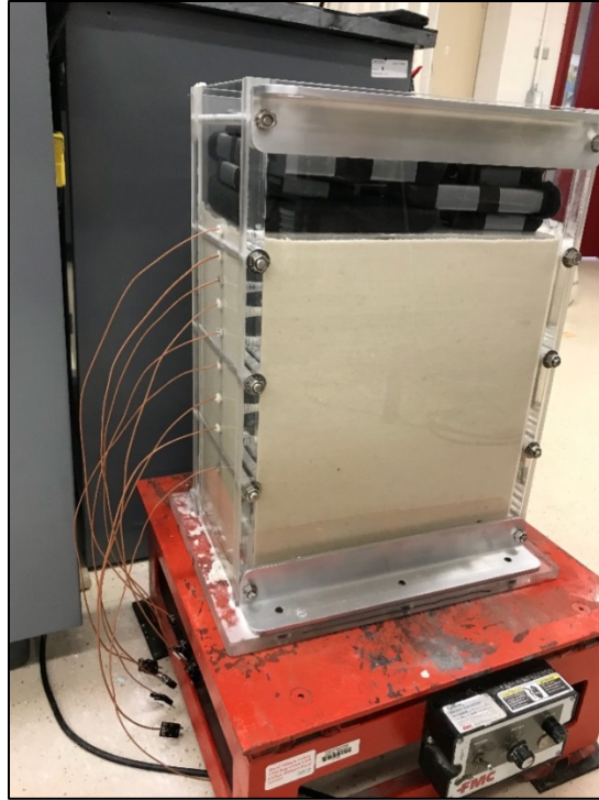
Figure F-7: Vibratory compaction of the sand in the column.
