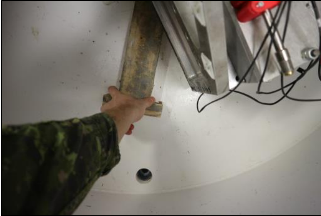
Figure D-57: Removal of wooden stand from the centrifuge casing.
