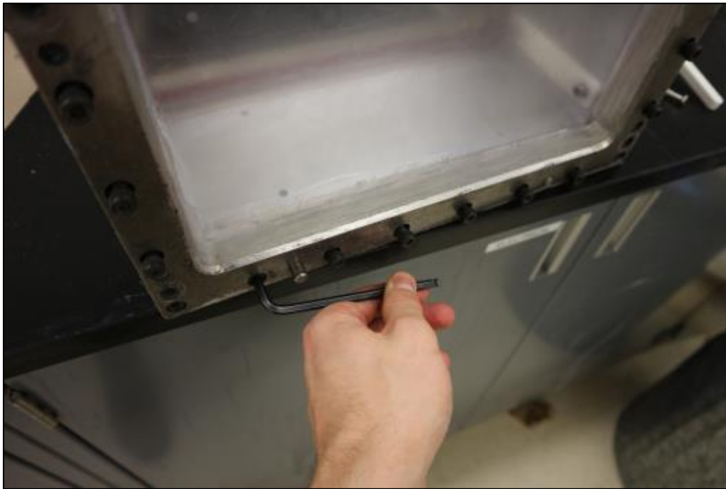
Figure D-24: Tightening capscrews.
