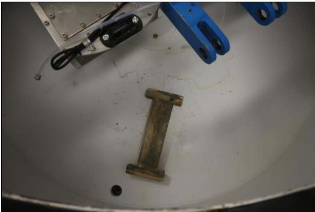
Figure D-50: Wooden stand placed at the bottom of the centrifuge casing.
