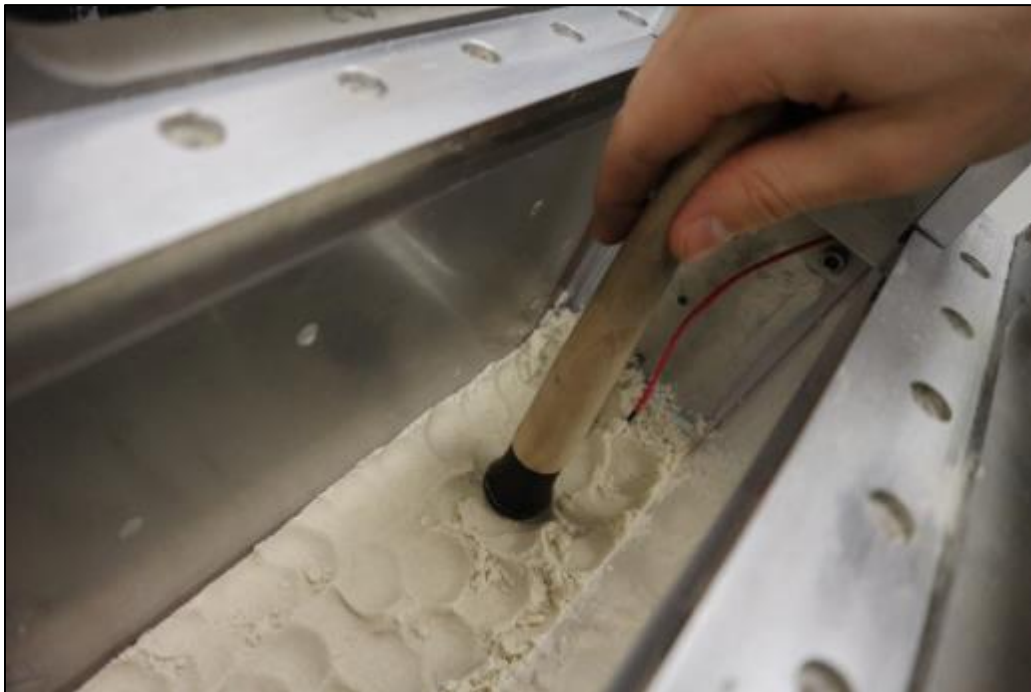
Figure D-36: Compaction of sand in the cradle.
