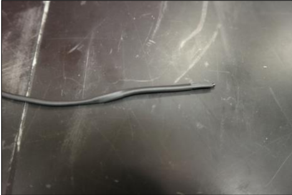
Figure E-9: Heat shrink tubing installation.
