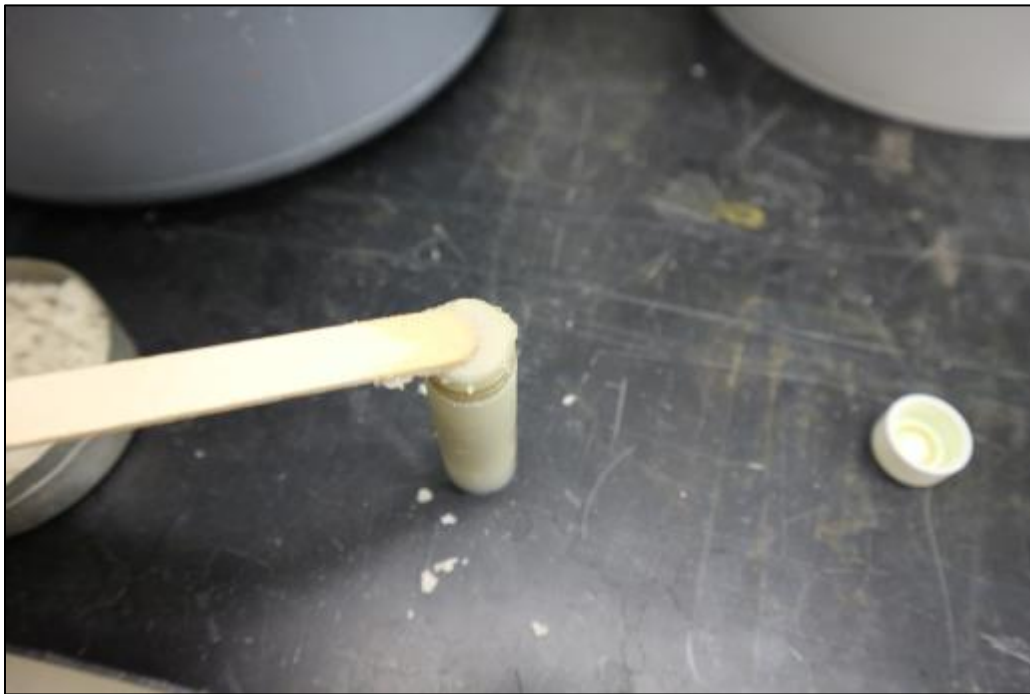
Figure D-45: Adding sand to fill the gap in the oil vial.
