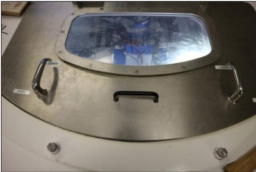
Figure D-80: Placing centrifuge casing lid handles into the locked position.
