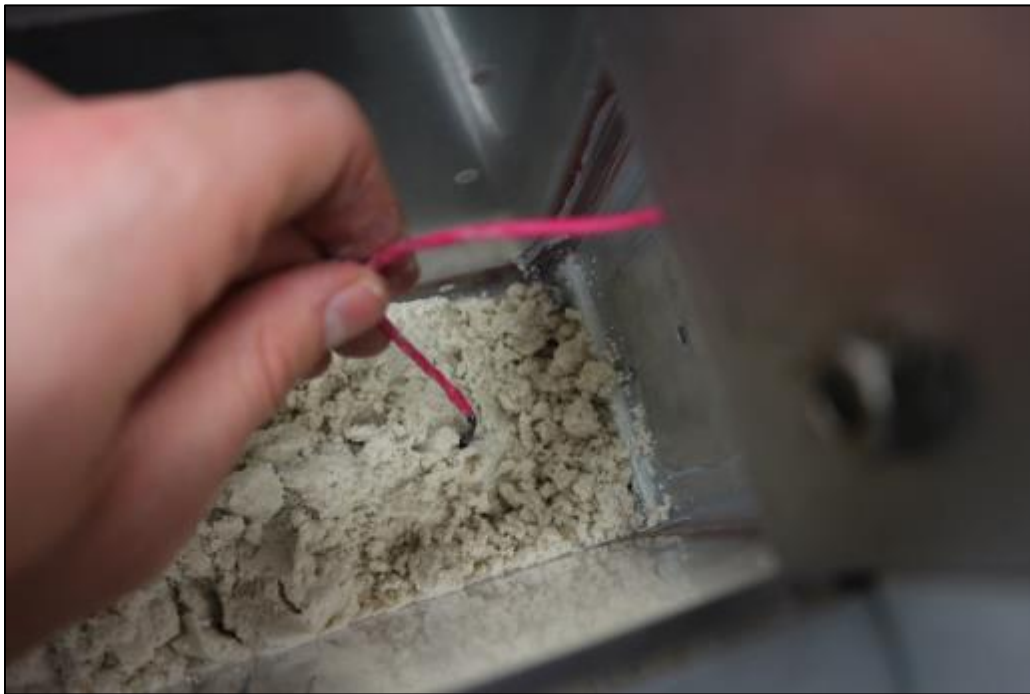
Figure D-39: Inserting the thermistor in the sand prior to compaction.
