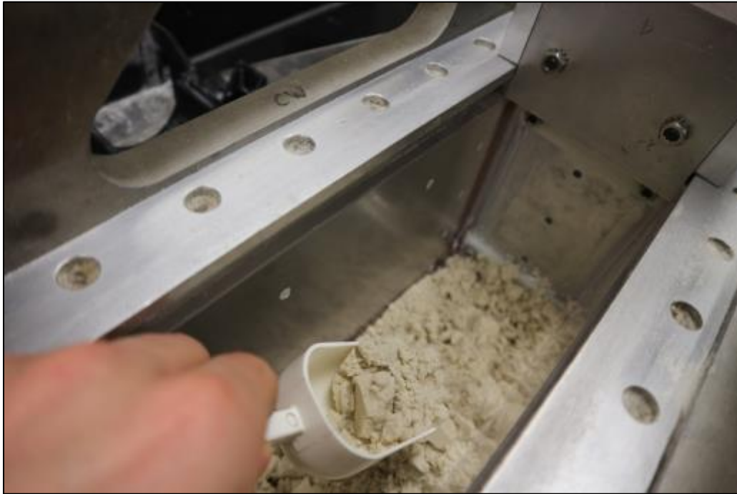
Figure D-35: Adding sand and water mixture to the cradle.
