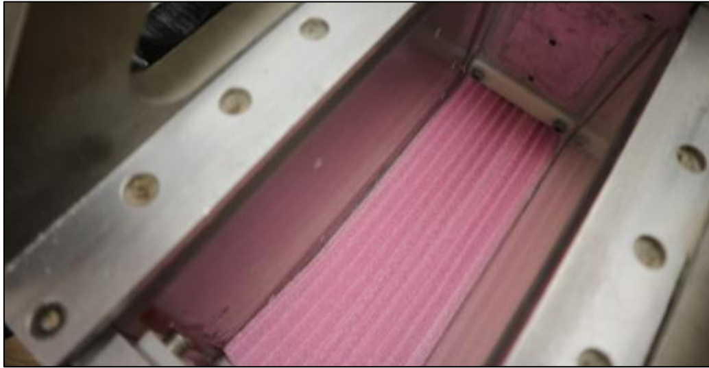
Figure 3-25: Foam insulation at the bottom of the centrifuge cradle.
