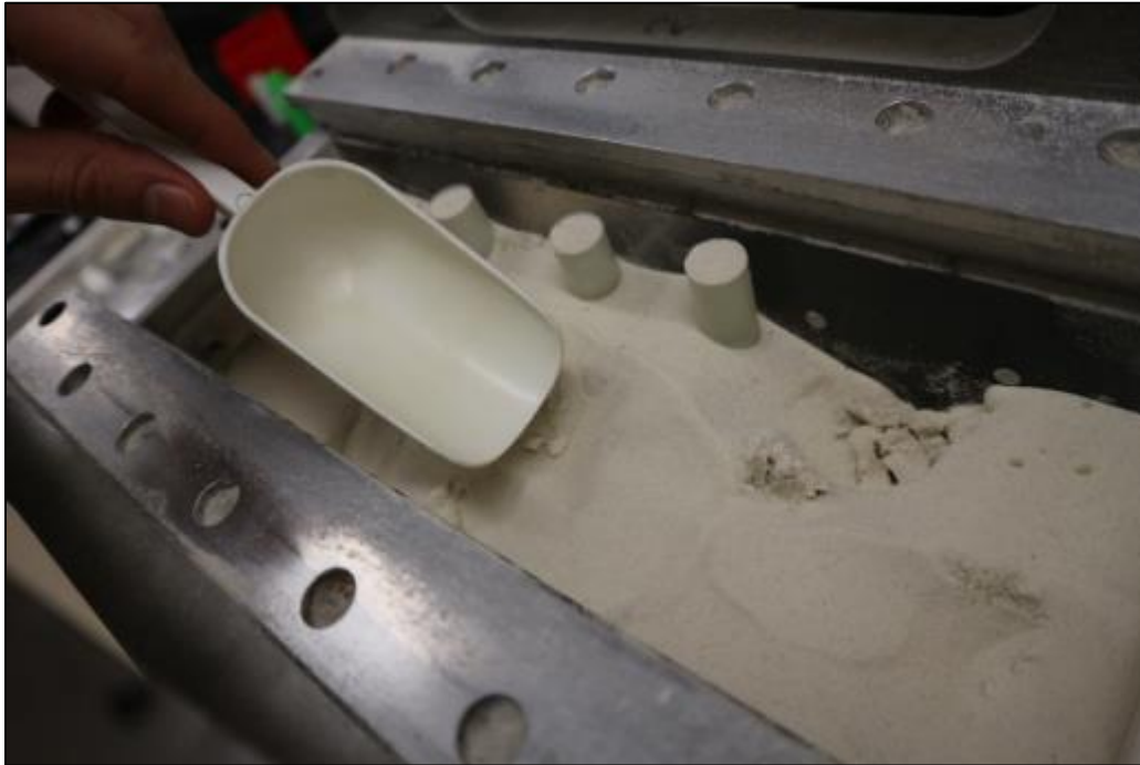
Figure D-100: Collecting soil to measure the water content throughout the sample.
