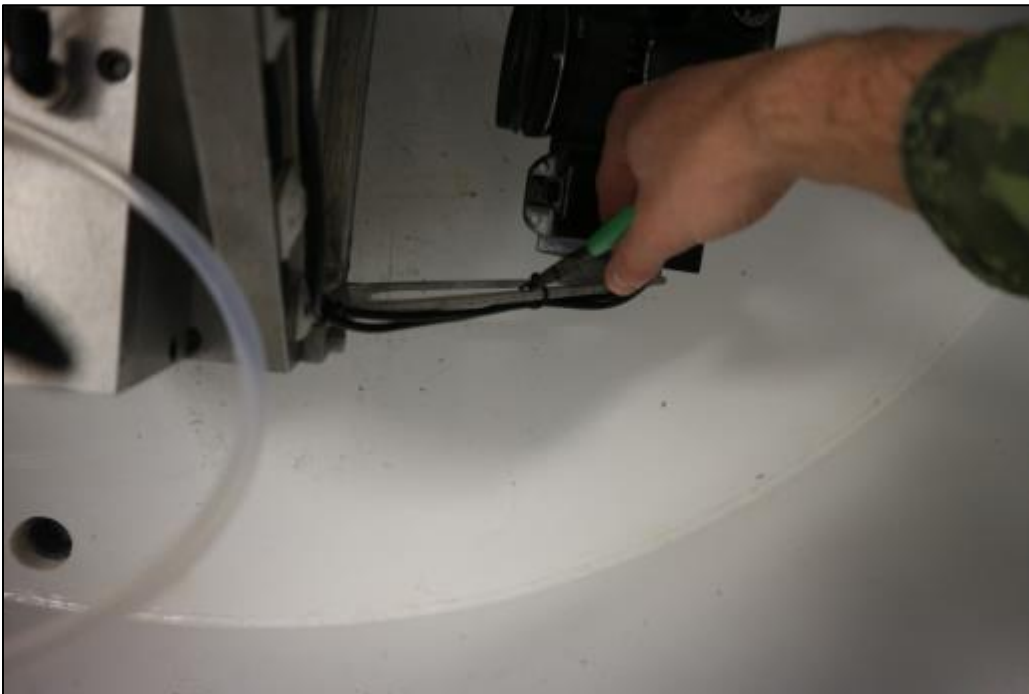
Figure D-98: Cutting the zip ties securing the camera wires.
