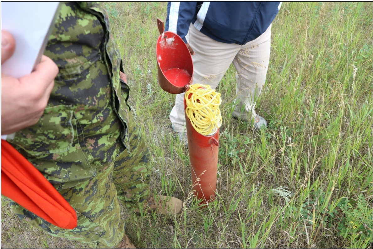
Figure F13 - Bailer rope obstructing a MW lid and filling the casing cavity (SL#8).
