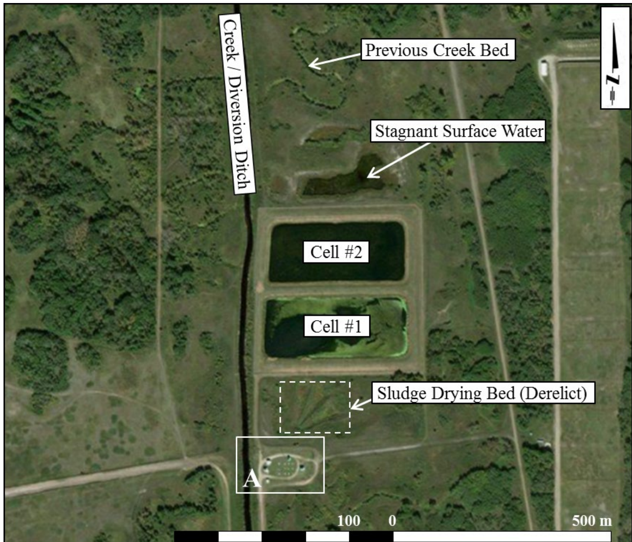
Figure D1 - Points of interest at the WWT lagoon site (Imagery provided by Microsoft Corporation 2018)
