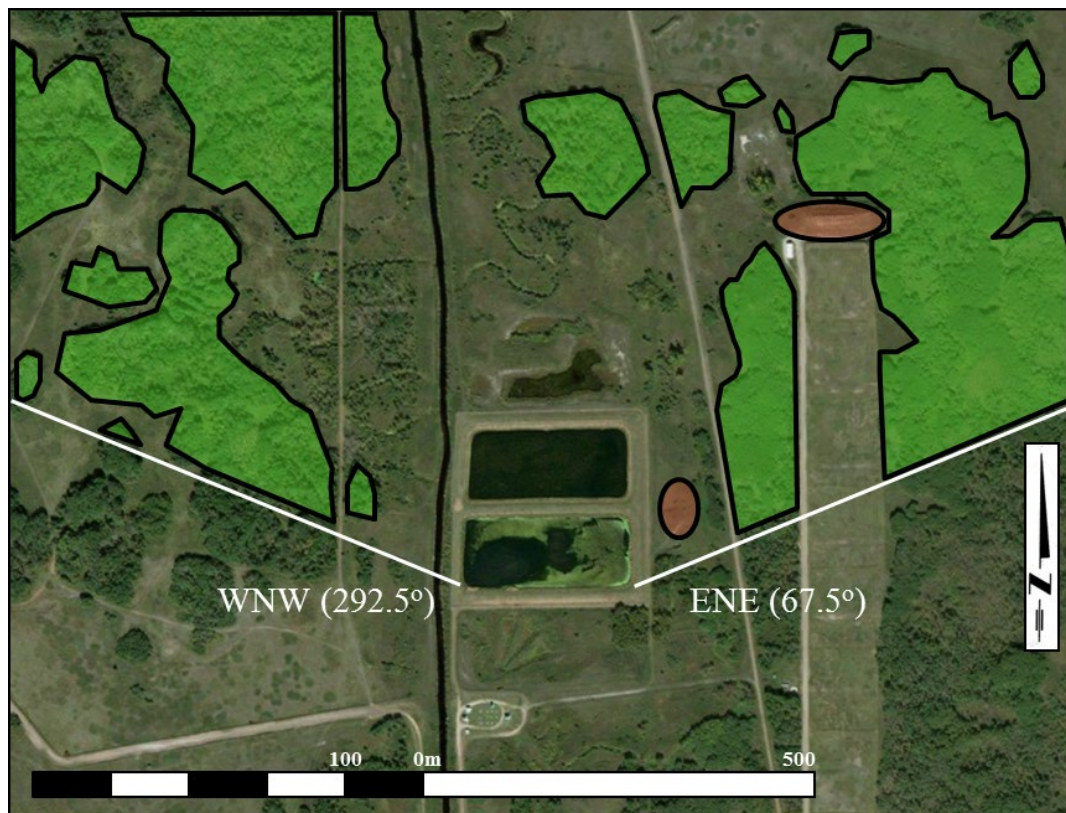
Figure 8.2 - Obstacles to wind
