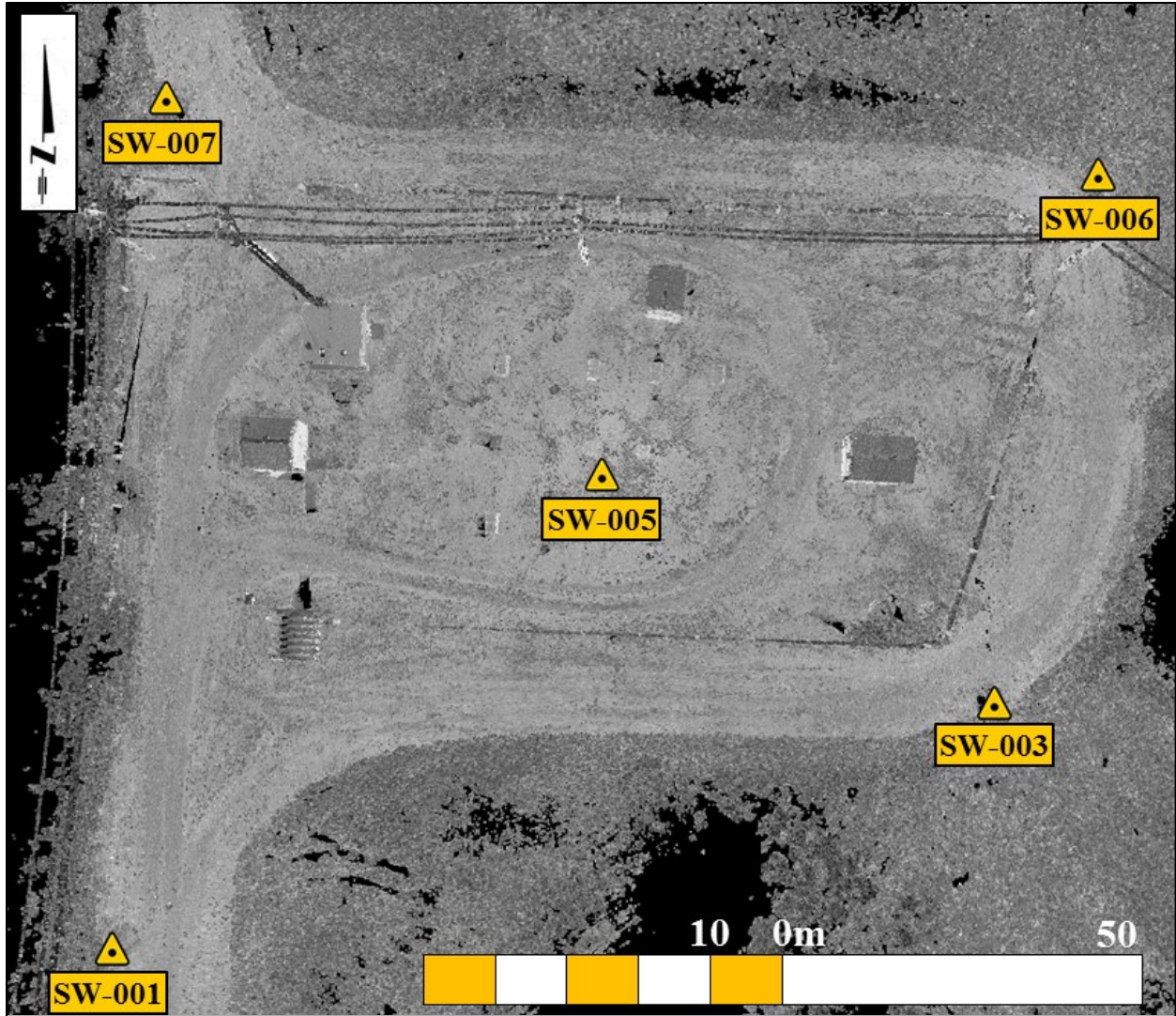
Figure I4 - Scan station layouts conducted in AOI 2
