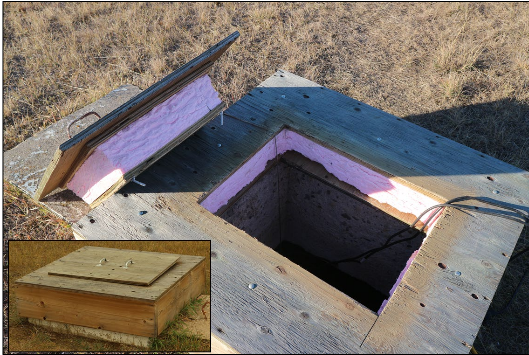
Figure 5.1 – Septic tank sampling point with a submersible pump in operation
