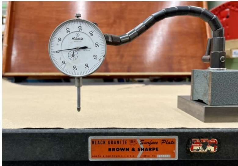
Figure 4.8: Dial indicator (distance amplifying instrument) with spherical tip on flat surface used to measure dent depth.
