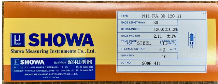
Figure A.2: Manufacturer's Certificate, Strain Gauge Type N11-FA-30-120-11 Lot 9008-411.
