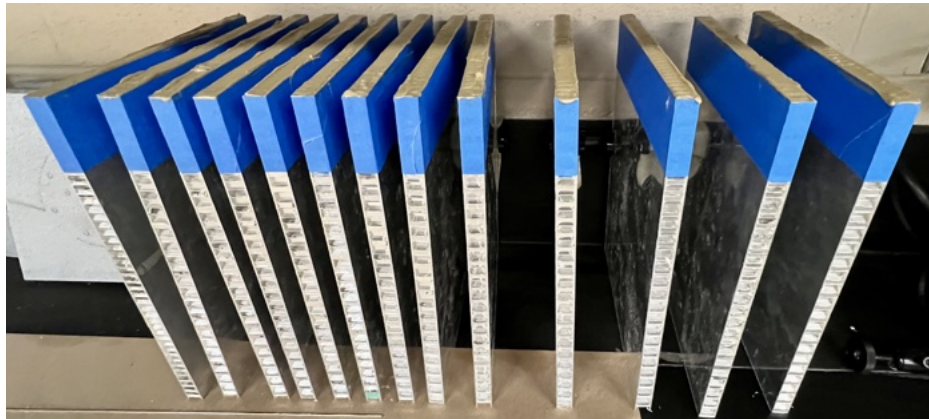
Figure 4.4: Test panel top edges have been filled with construction adhesive and are curing.
