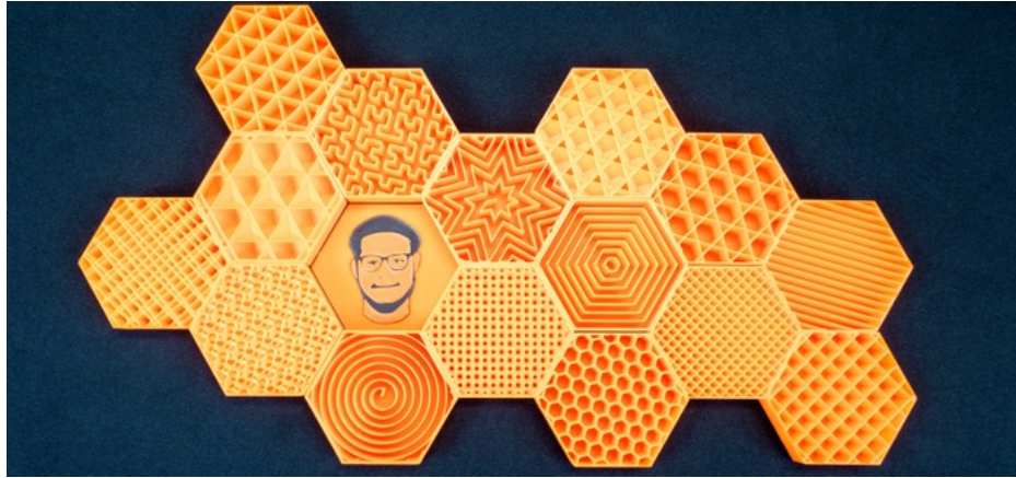
Figure 2.2: Various 3D printed part infill patterns are used to provide structural support to outer layers of filament-printed components. Infill patterns, like more traditional sandwich core materials, are normally selected based on design needs [19].
