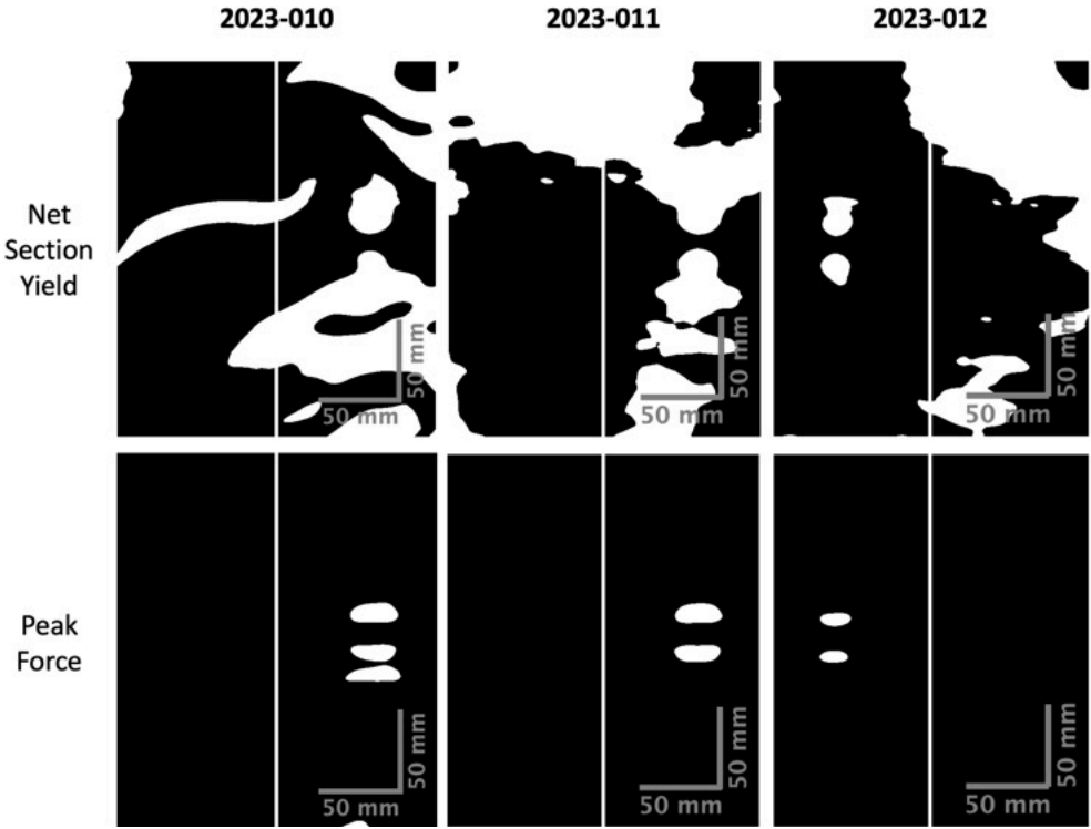
Figure 5.17: 50 mm ED dent strain. Black identifies area in plastic strain while white identifies areas under elastic strain. Scale bars are 50 mm. The vertical white line marks the panel centre.
