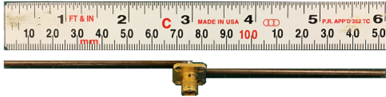
Figure 4.19: Fabricated half-wavelength dipole antenna operating at 1 GHz using copper rods with diameter of 1 mm where the total antenna length is 152 mm. The wires are both linked through an SMA-50 \Omega connector.
