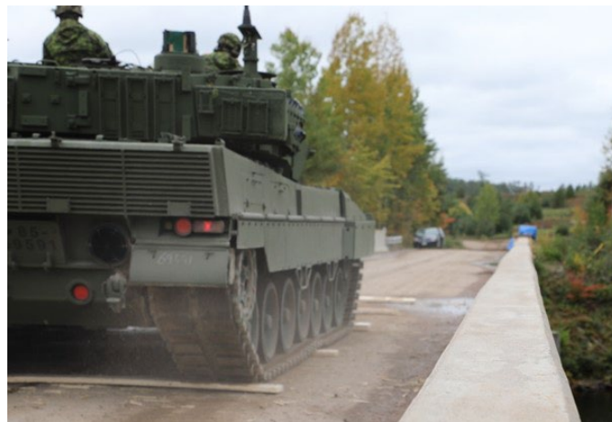
Figure 4-12. Leopard 2 travelling over a series of five 38 mm tall obstacles spaced 3.0 m apart.
