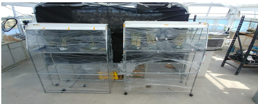
Figure 4-1 Covered plant stands. The plants were rinsed, watered, and placed inside the stands for one week prior to imaging by SEM. The stands were encased with plastic wrap to prevent air disturbances. A grow light on a 12-hour cycle was provided to assist with growth and salt excretion. The conditions in the stands were considered optimal with relative humidities of 55-65% and temperatures of 22-26 °C.
