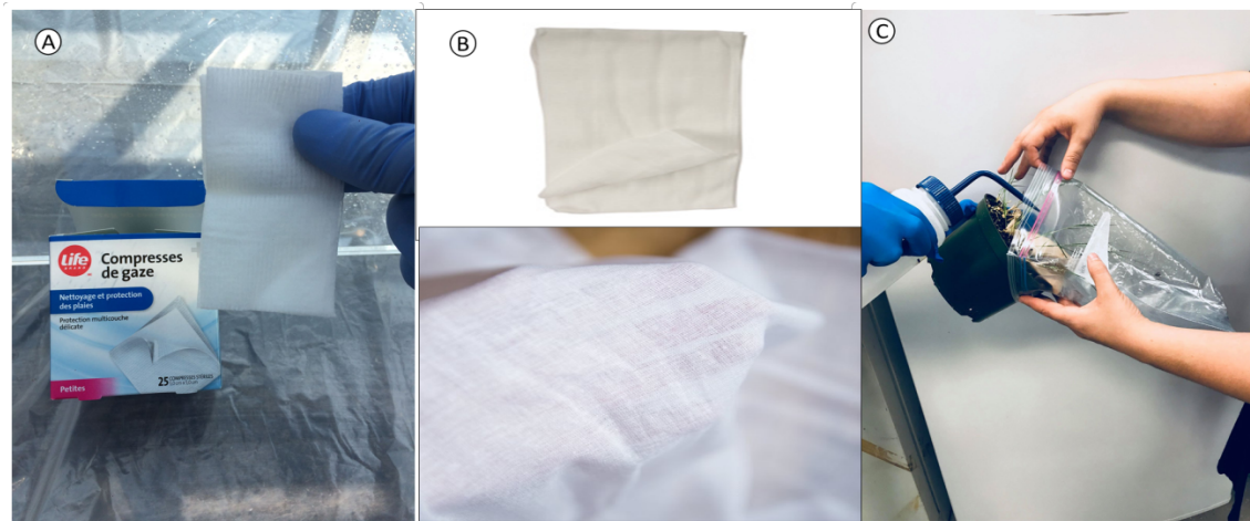
Figure 5-3 Salt was collected from within the wind tunnel by; (A) swabbing the inside at 30 cm increments, (B) capturing it in tightly woven grade 80 cheesecloth that allowed air to pass through while trapping salt in its fibres, and (C) rinsing any remaining salt off of the plant.
