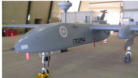
Figure 1.1.2: The C170 Heron is a medium-altitude long-endurance UAV used in Afghanistan [2].
