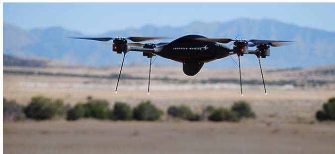
Figure 1.1.4: Lockheed Martin Indago is a UAV capable of VTOL for short range ISR type missions [4].
