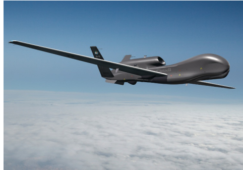
Figure 1.1.1: The Northrop Grumman RQ-4 Global Hawk. An example of a UAV for long range, high altitude ISR missions [2].
