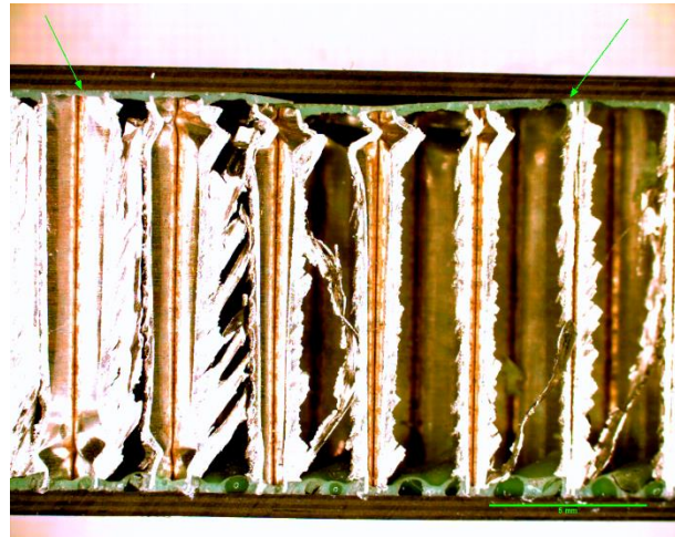
Figure 95: Test Panel 1 (5 Ply, [0/90/0/90/0]) 0.7357 J Impact. Thermography measured width = 25.8 mm (Left), Microscope measured width = 15.3 mm, Microscope measured core crush depth = 0.37 mm (Right).
