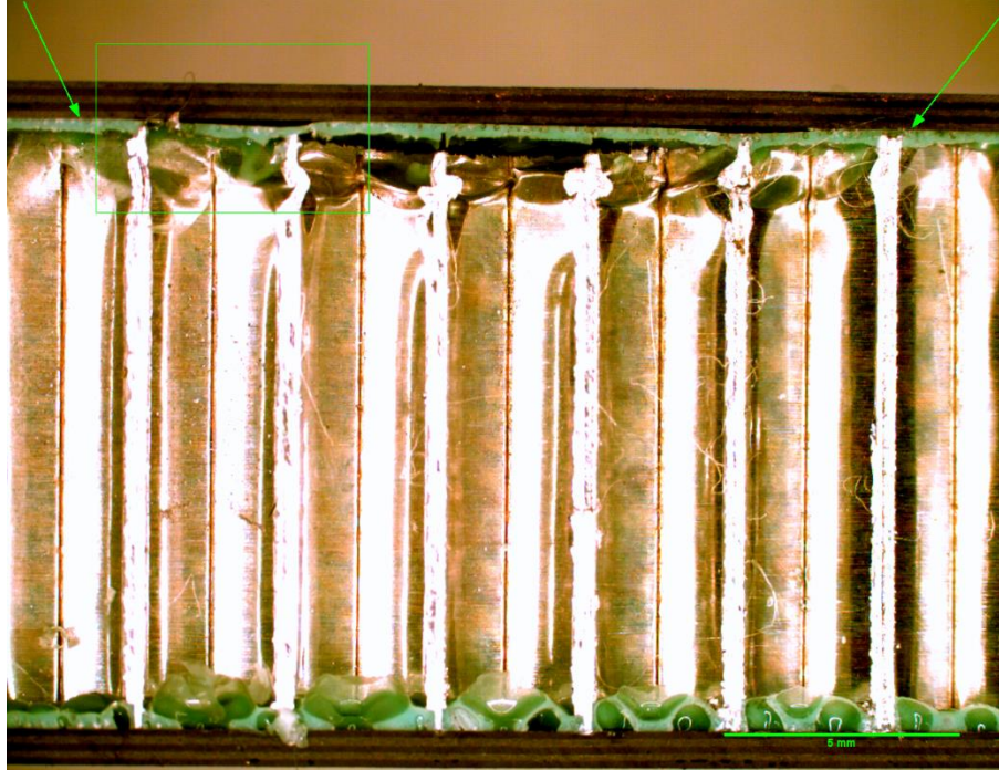
Figure 64: Test Panel 1 (5 Ply, [0/90/0/90/0]) Impact energy of 0.88 J. The green arrows point to where the disbond visually starts and the green box is looked at in more detail in Figure 65. (6.3x zoom) (Scale Bar = 5.0 mm)
