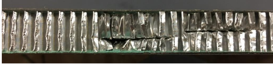
Figure 37: Horizontally sliced honeycomb core. This was created by pushing an X-Acto knife blade into the side walls of the cells.
