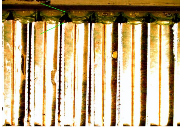
Figure 85: Test Panel 11 (5 Ply, [0/-45/90/+45/0]) Impact energy of 0.88 J. The green arrows point to where the honeycomb core has become unbonded from the film adhesive, leaving a small void.
