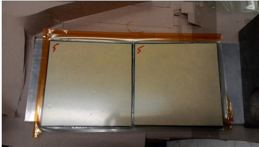
Figure 22: Two face sheets (5 ply, [0/90/0/90/0]) vacuum pressed together and ready for curing.
