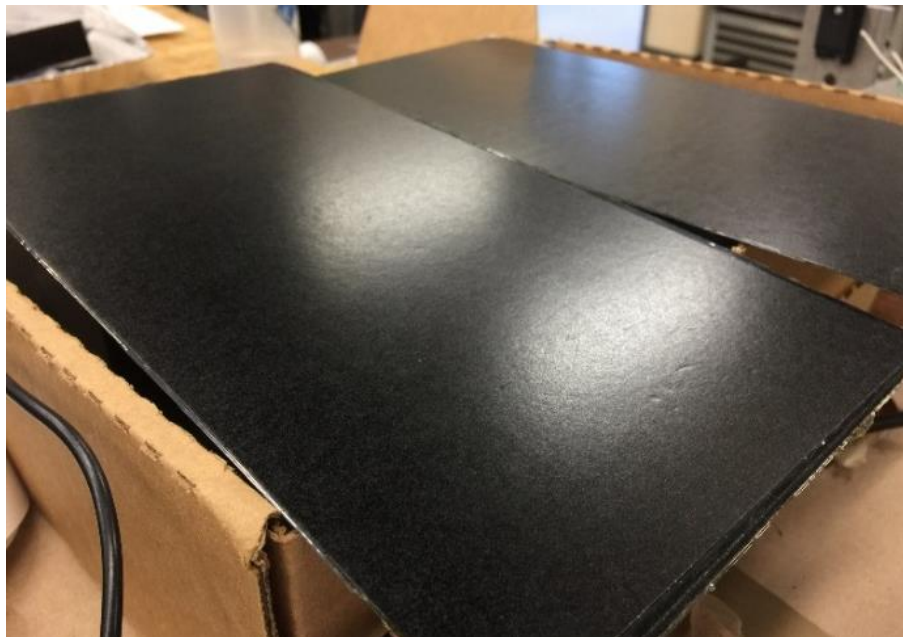
Figure 24: Two 152 mm x 305 mm (6.0 inch x 12 inch) (5 ply, [0/90/0/90/0]) post-cured face sheets.
