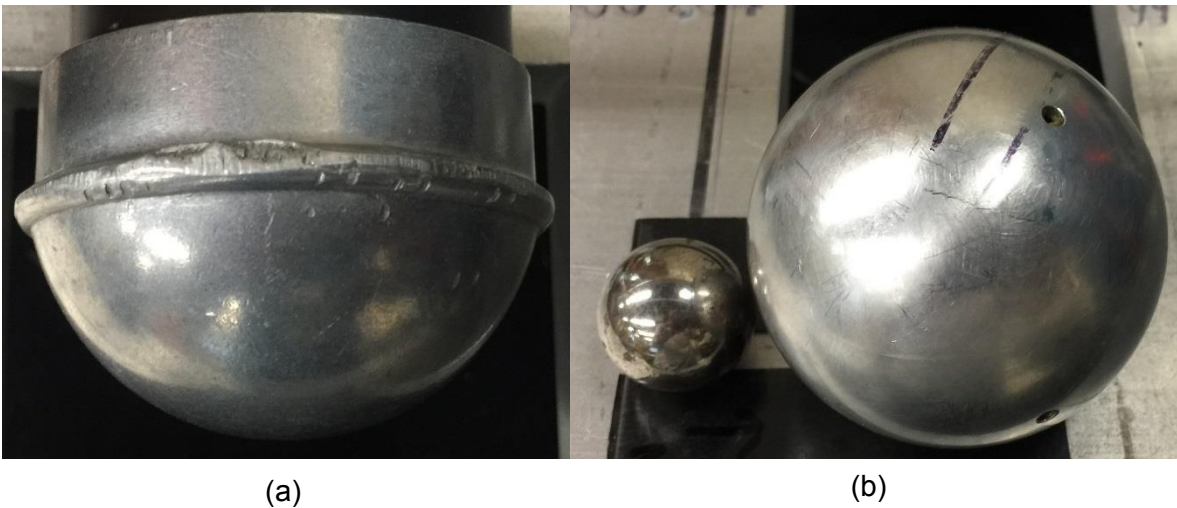
Figure 28: (a) Impactor 1 with a mass of 0.150 kg, and a diameter of 52.6 mm. (b) Impactor 2 with a mass of 0.067 kg and a diameter of 25.4 mm and impactor 3 with a mass of 1.030 kg and a diameter of 63.1 mm.
