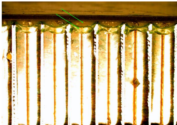
Figure 82: Test Panel 11 (5 Ply, [0/-45/90/+45/0]) The green arrows point to the two layers of film adhesive, which are able to absorb extra thermal energy.
