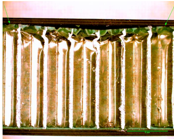
Figure 97: Test Panel 1 (5 Ply, [0/90/0/90/0]) 1.4715 J Impact. Thermography measured width = 27.4 mm (Left), Microscope measured width = 18.8 mm, Microscope measured core crush depth = 0.56 mm (Right).
