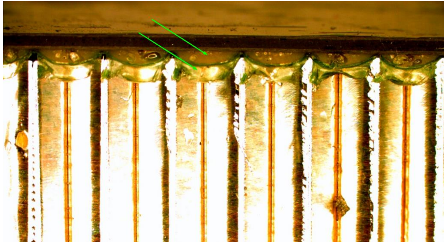
Figure 34: Excess adhesive created by adding an extra layer (Green) of film adhesive before the curing process.
