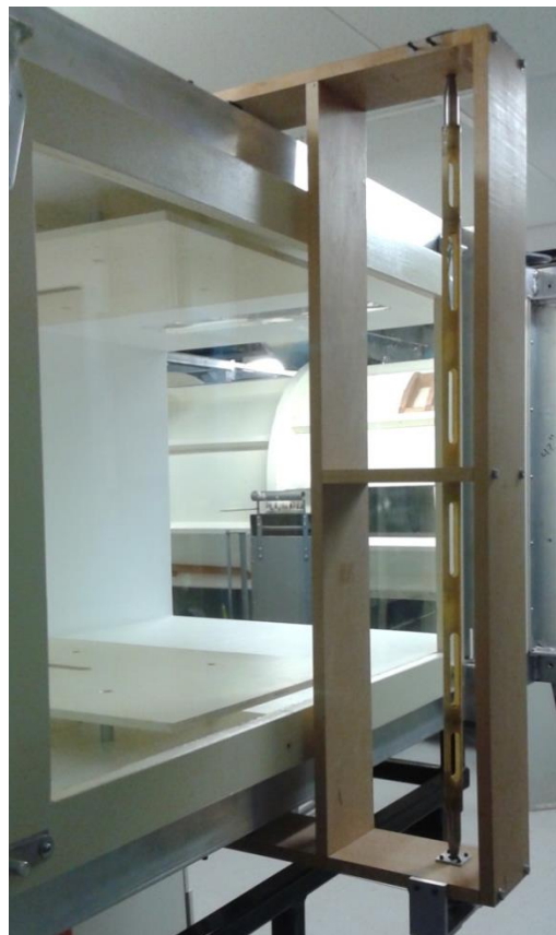
Figure 2.4: External rod on side of test section connecting heave spring/pulley systems
