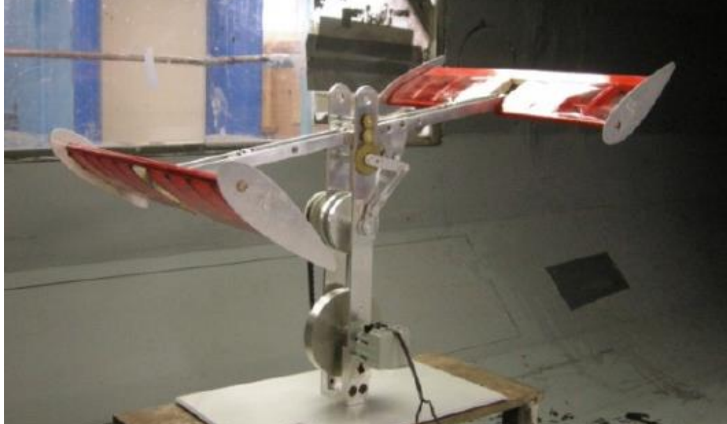
Figure 1.6: The reciprocating tandem-wing experimental prototype in the wind-tunnel at Laval University. Taken from [9].
