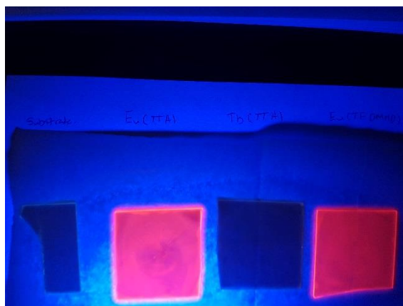
Figure 10: Fluorescent behaviour of spin coated samples of the two europium(III) complexes via irradiation with UV light. From left to right: untreated substrate, Htta europium(III) complex, 68a•Eu(III) , Htta praseodymium(III) complex, 68a•Pr(III) , and Hfdh europium(III) complex, 68b•Eu(III) .
