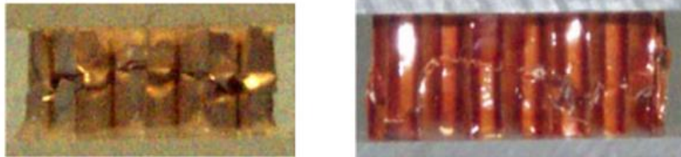
Figure 5-5: Comparison of crushing behaviour of compacted aluminum and Nomex™ honeycomb cores [Adapted from Reference 28]
