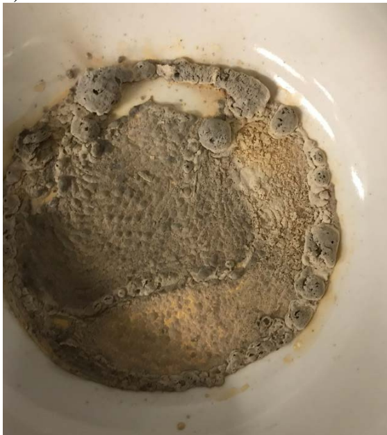
Figure 4.31 SCS a) \text{CaMoO}_4 and b) \text{SrMoO}_4 products that just came out of the muffle furnace.
