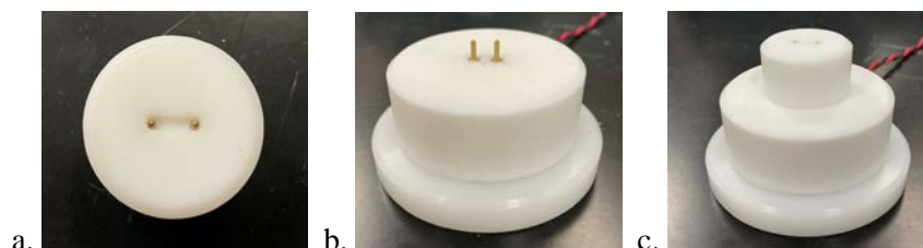
Figure 2.3. Resistivity measurement apparatus. a) Sample cell b) base unit c) cell base arrangement.
