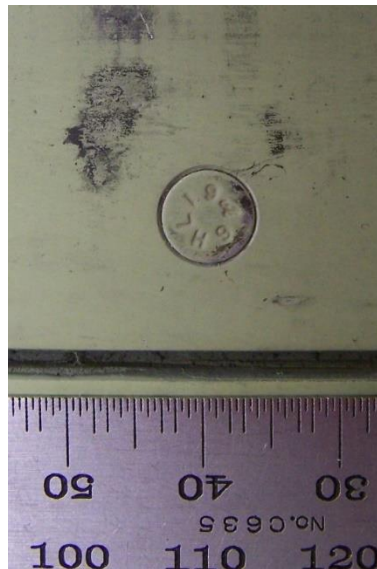
Figure 45: Image of fastener 24 on NAVAIR Standard 23 showing surface damage.
