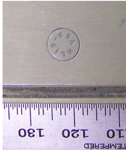
Figure 26: High resolution image used for fastener to lap-joint edge distance measurements.
