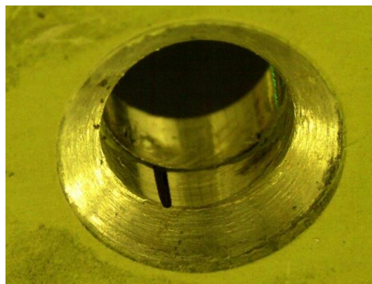
Figure 29: Laser image of hole 18 on Standard 26 displaying an 0.080" notch located at the bottom of the top layer, oriented at 225° CW from the lap-joint edge.
