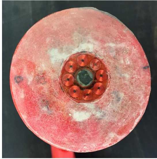
Figure 16: Face of PEC probe utilized in experimental data collection showing 8 mm ferrite core surrounded by array of eight pick-up coils.
