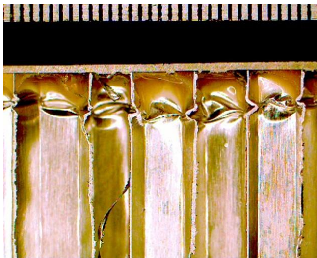
Figure 1.4: Side view of a sectioned panel with impact damage [2].
