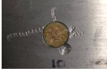
Figure 2: Typical damage that can occur to wing skin during fastener removal.
