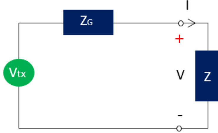
Figure 3.4 Circuit equivalent for radar transmit array.
