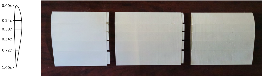
Figure 6.9: 3D printed monocopter blade cross section, and blade segments with rectangular tabs ready for final assembly.
