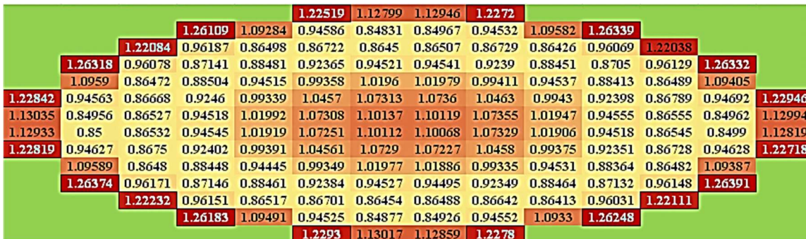
Figure (7-49): Power Density Distribution in the Fast Core of MSCR-Model (II) after 1000 Days. (The power density units are in W\text{ cm}^{-3} )
