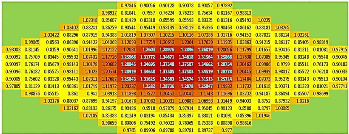
Figure (8-28): Power Density Distribution in the Fast Core after 2600 Days for the MSCR- Model (IV) (The power density units are in W\text{ cm}^{-3} )
