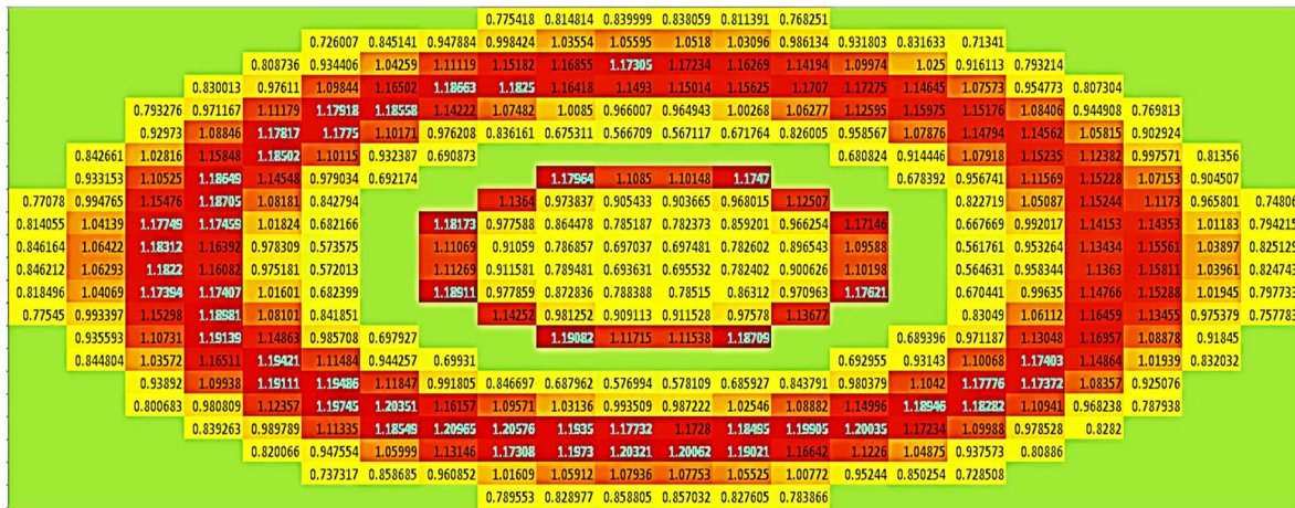
Figure (8-21): Power Density Distribution for the Freshly Fueled Core of the MSCR-Model (III) (The power density units are in W\text{ cm}^{-3} )
