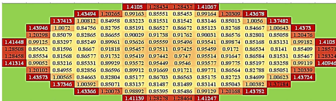
Figure (7-47): Power Density Distribution for the Freshly Fueled Fast Core of MSCR-Model(II) (The power density units are in \text{W cm}^{-3} )
