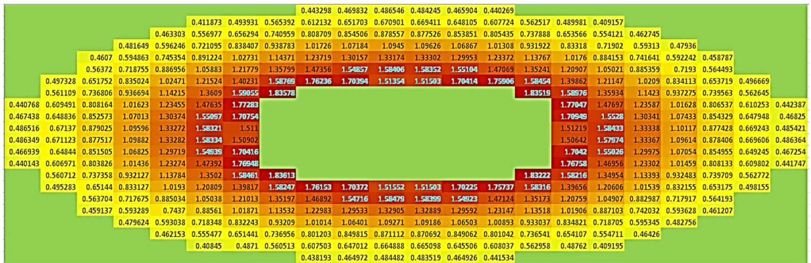
Figure (8-30): Power Density Distribution for the Freshly Fueled Thermal Core of the MSCR-Model (V) (The power density units are in W\ cm^{-3} )
