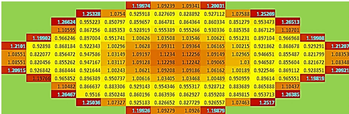
Figure (8-33): Power Density Distribution in the Fast Core after 1060 days of the MSCR Model (V) (The power density units are in W\ cm^{-3} )
