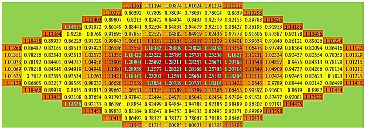
Power Distribution in the Thermal Core and Fast Core of MSCR-Model (IV) after (4 days)
