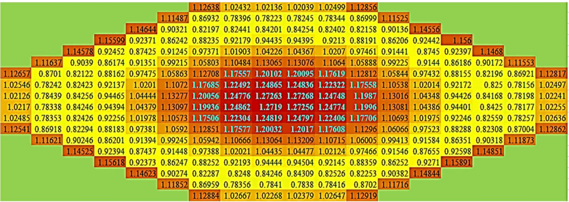
Power Distribution in the Thermal Core and Fast Core of MSCR-Model (IV) after (0.5 day)
