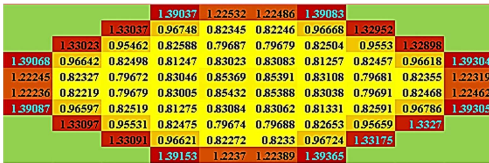
Figure (8-39): Power Density Distribution for the Fast core after 420 days of the MSCR Model (VI) (The power density units are in W\ cm^{-3} )
