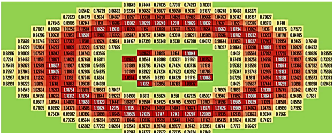
Figure (7-27): Power Density Distribution in the MSCR Core after 150 Days of the MSCR-Model (I) (The power density units are in \text{W cm}^{-3} )
