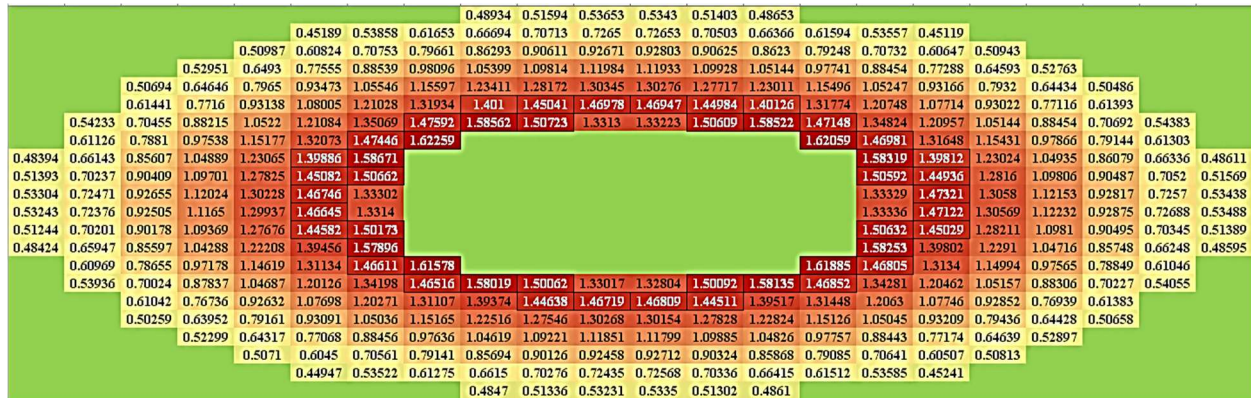
Figure (7-46): Power Density Distribution for the Freshly Fueled Thermal Core of MSCR-Model(II) (The power density units are in \text{W cm}^{-3} )
