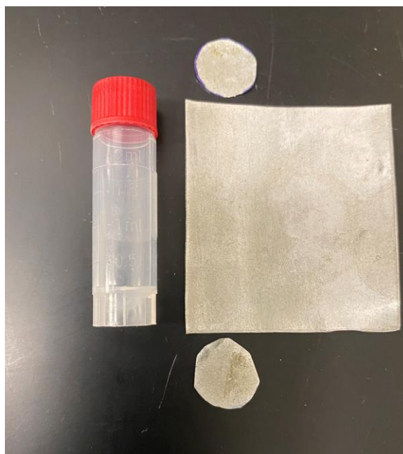
Figure 27. 2 mL Vial (Left) and its Prepared Cadmium Shield (Right)
