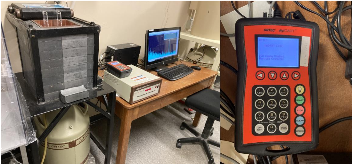
Figure G-2. General Arrangement of the HPGe Detector and Associated Equipment at the RMC
