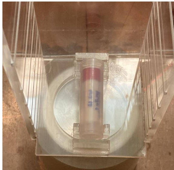
Figure H-3. Sample on the Detector Sample Holder's First Step Undergoing Detection on the HPGe
