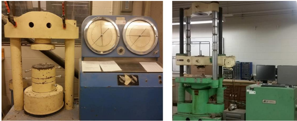
Figure 4.4: Material Testing Systems. Left; RIEHLE Compression Machine. Right; Baldwin Universal Testing Machine
