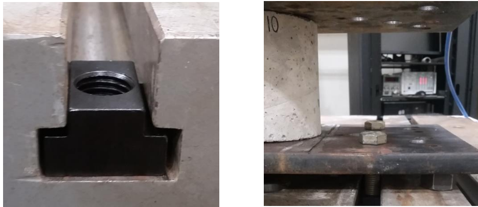
Figure 5.10: Left: T-nut in MTS T-slot platen. Right: Fixed attachment steel plate
